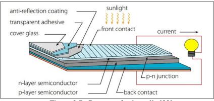
Figure 2.7: Concept of solar cells [32]
