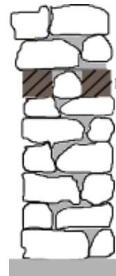
Figure 4.11: Masonry wall with horizontal timber ties (by author)
