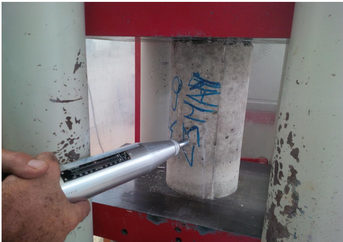
Figure 24: Schmidt Hammer Test
