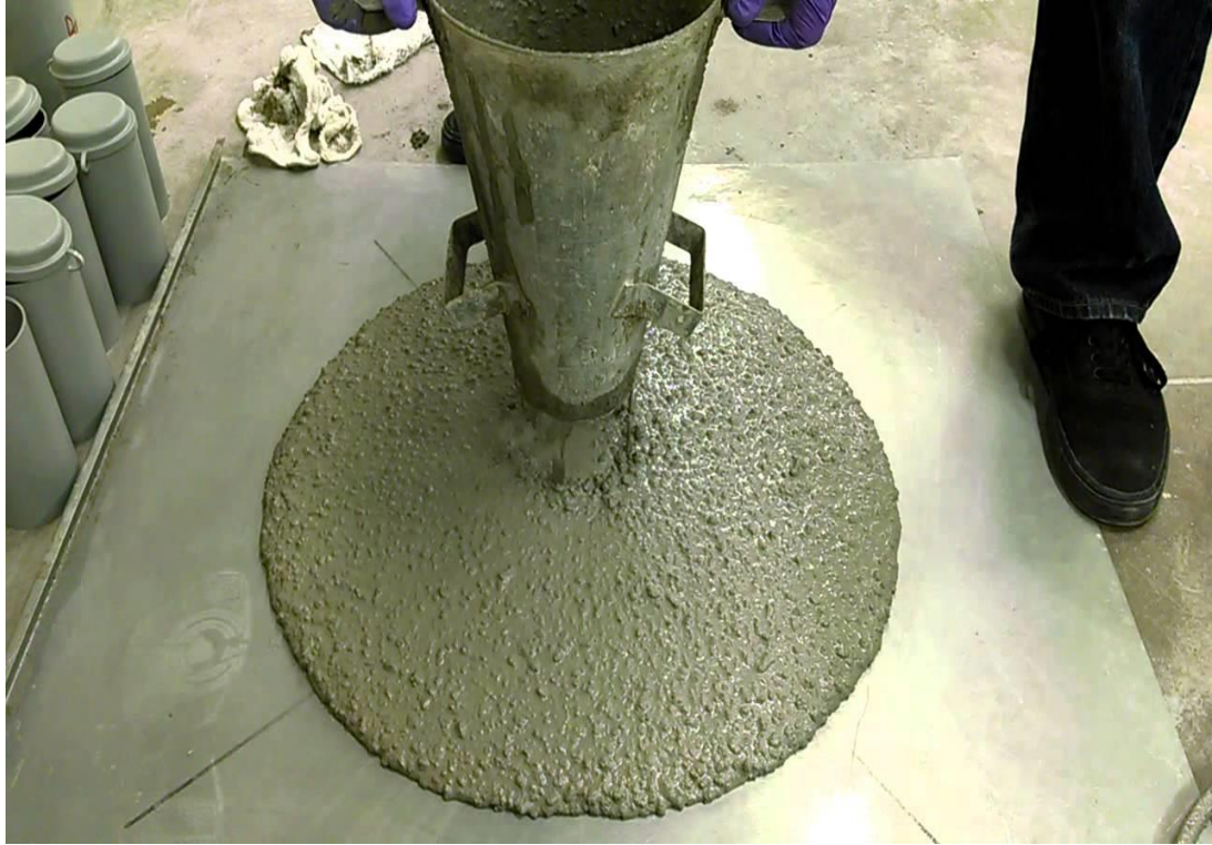
Figure 17: Slump test for SCC Mix
