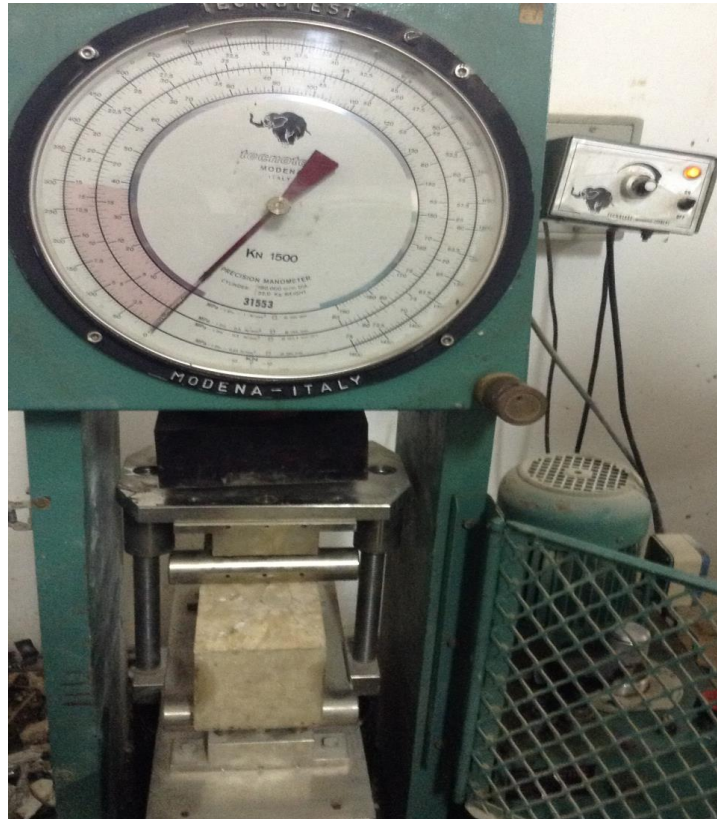
Figure 21: Flexure test by four-Point loading
