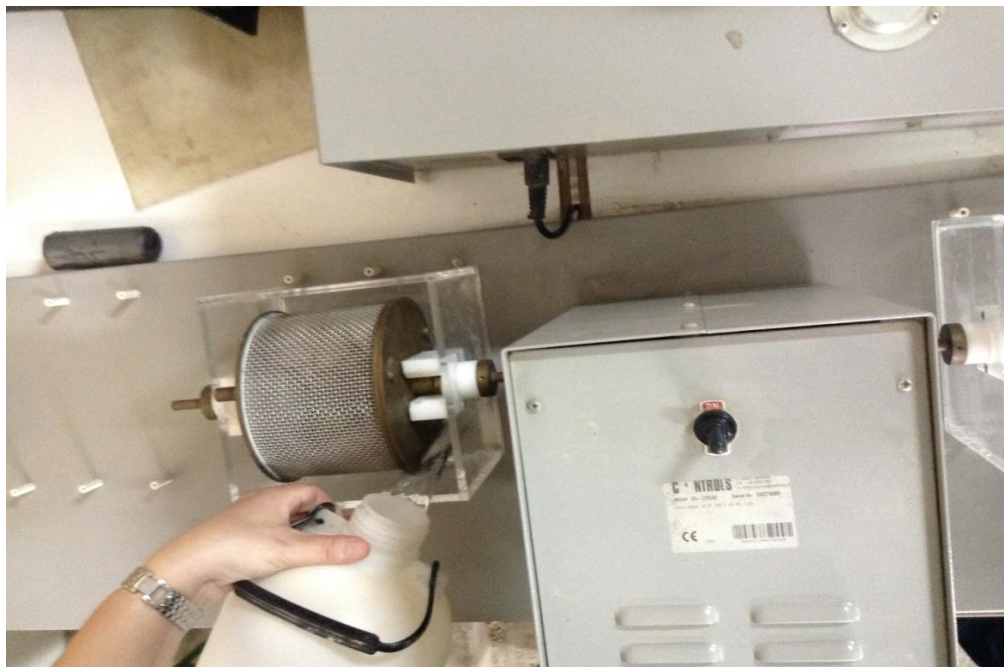
Figure 23: Adding distilled water to the tank of the slake durability device
