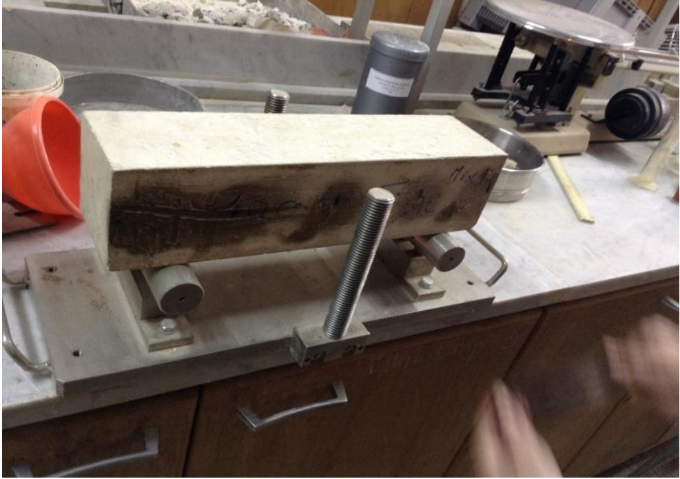
Figure 19: Beam under 4-points loading flexural test (a)
