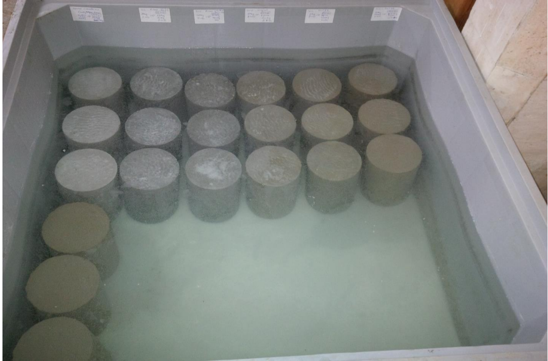
Figure 16: Test specimens in the curing tank
