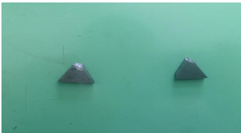
Figure 31: Broken Cutting tool from R9.
