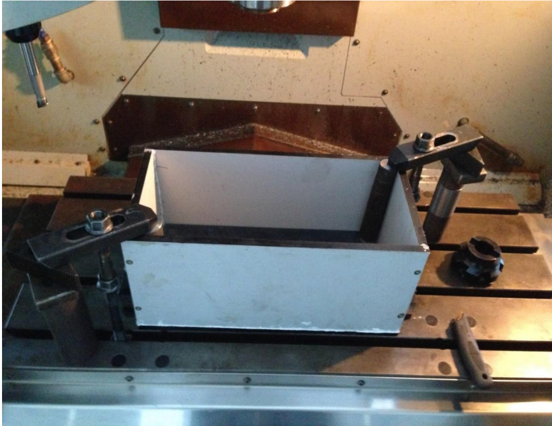
Figure 12: Fixtures used to hold still the work-piece.
