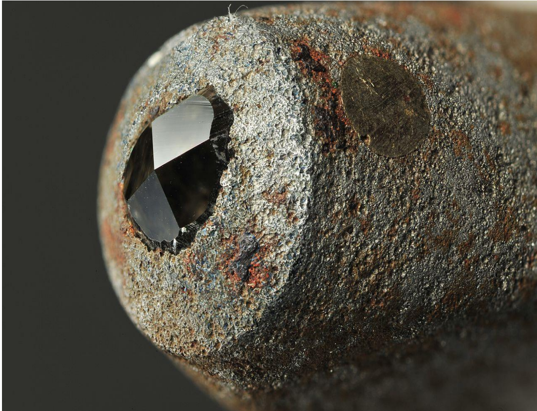
Figure 19: Indenter of a Vickers Hardness Tester, Pyramidal Diamond.
