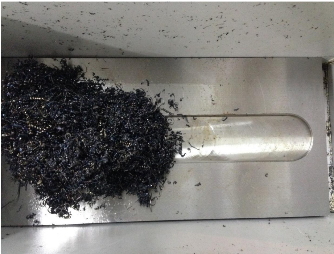
Figure 29: Formation of discontinuous chips affecting surface roughness.
