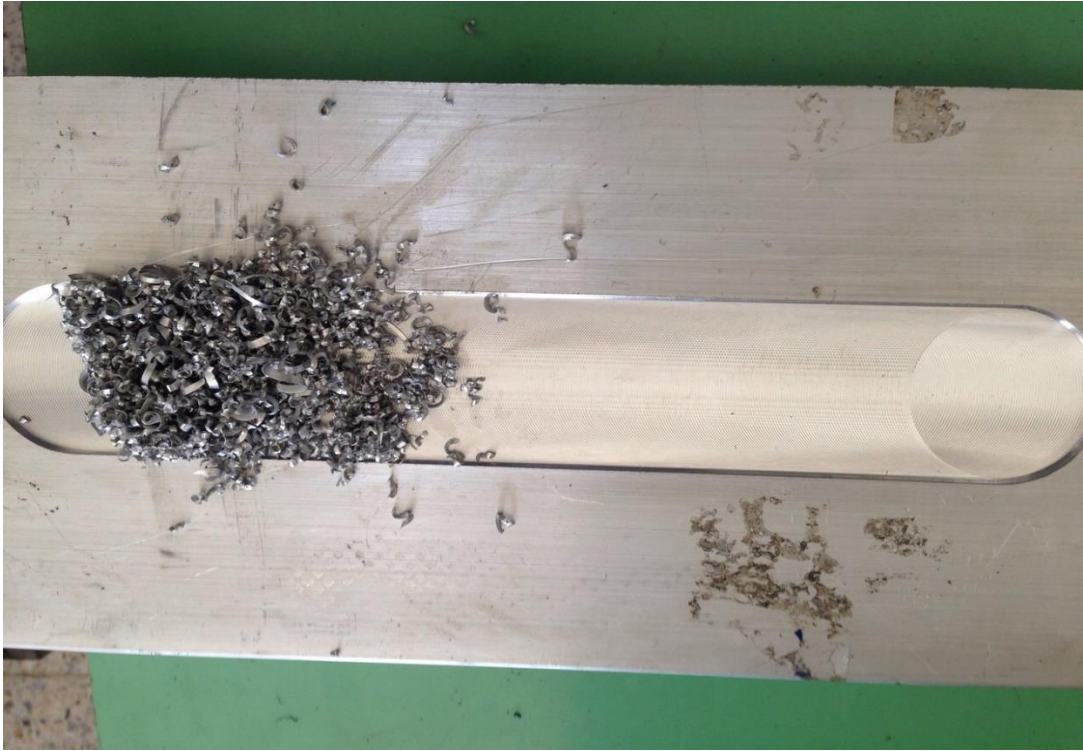
Figure 26: Irregular, thick, discontinuous chips.
