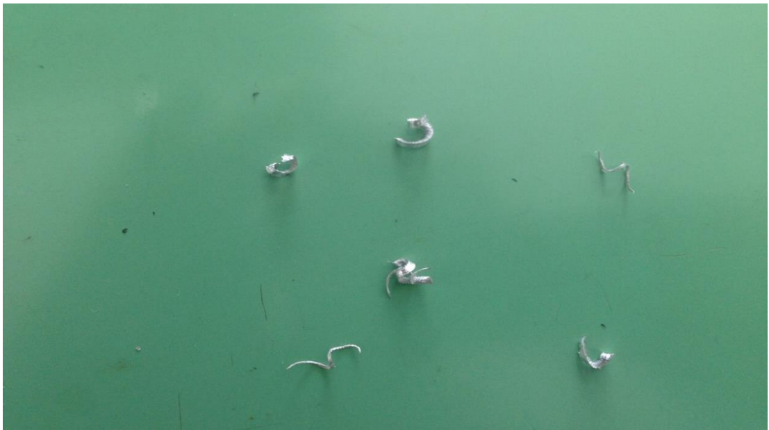
Figure 53: Chips formed from R9.
