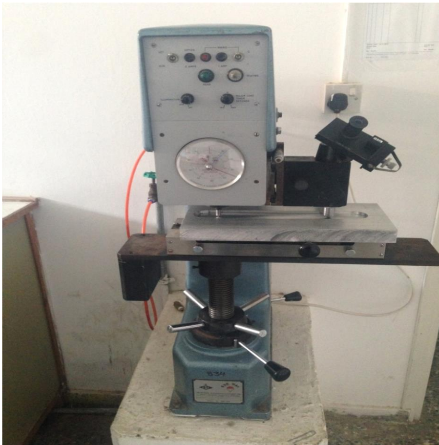
Figure 18: Device used for hardness test (indenting phase).
