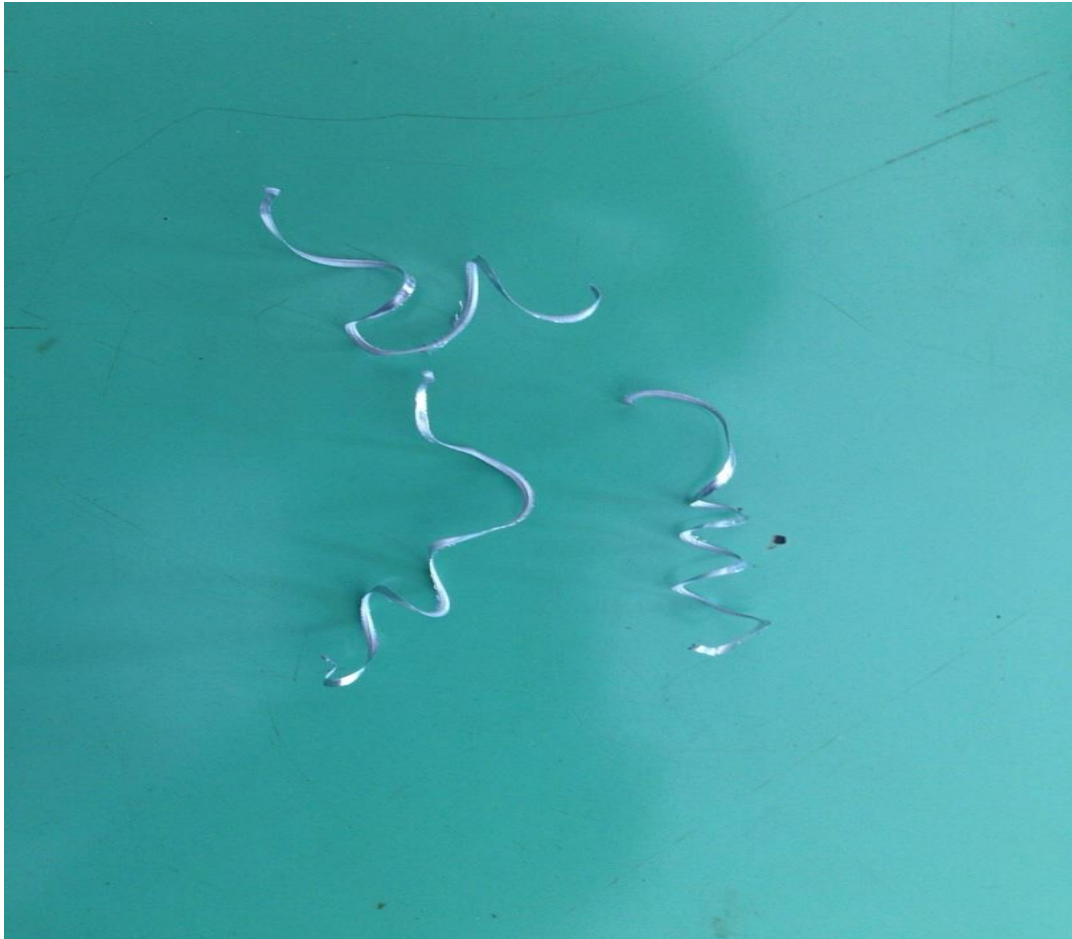
Figure 30: Example of smooth continuous chip formation.
