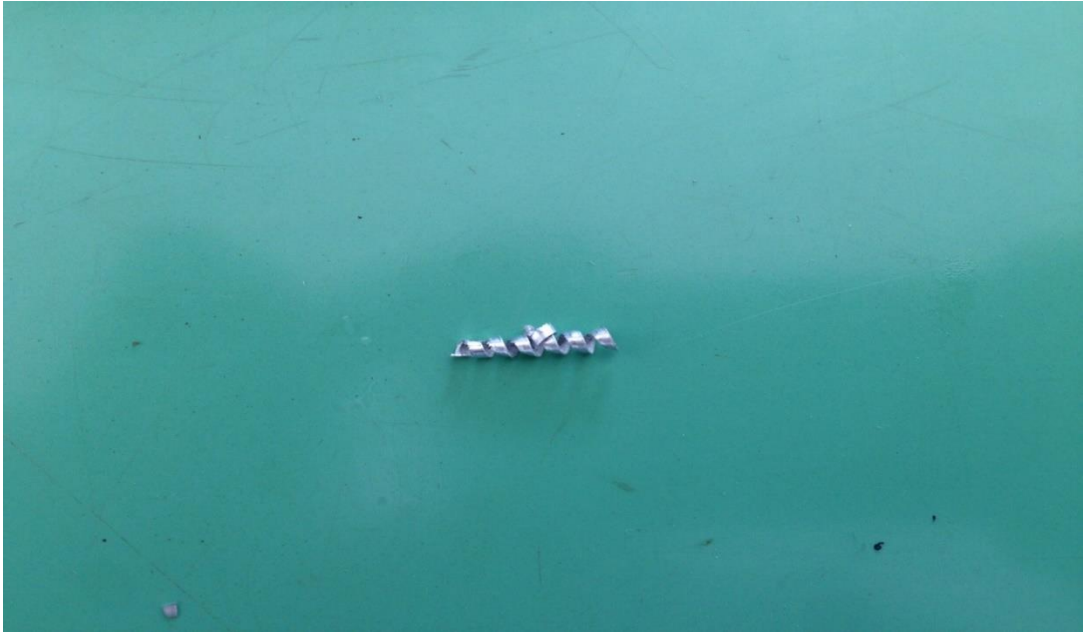
Figure 49: Chip formed from R8.
