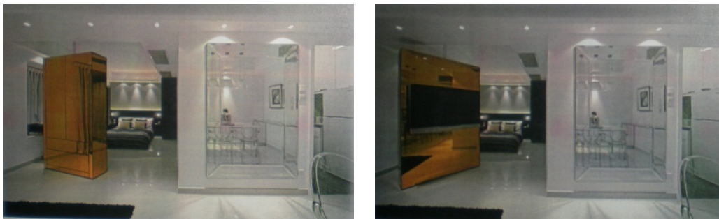
Figure 43: Rotation: A Bright Module That Turns on an Axis Can Change the Position of the TV And Separate the Two Rooms
