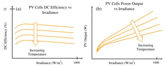
Figure 1. Temperature effect on PV cells: (a) efficiency; (b) power output [3]
