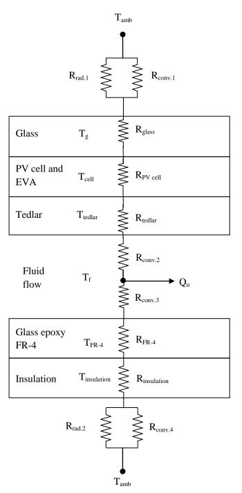
Figure 9. Thermal network of CPV/T collector
