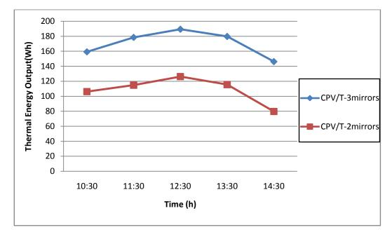
Figure 23. The CPV/T collector thermal energy outputs
