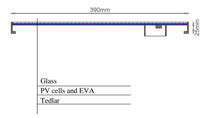
Section A-A Figure 3. Top and sectional view of the PV module
