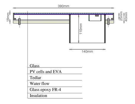
Section A-A Figure 4. Top and sectional view of the PV/T collector
