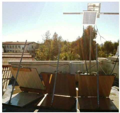
Figure 14. PV module and CPV/T collector setup
