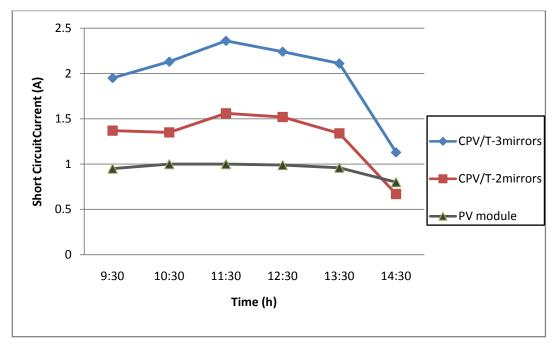
Figure 20. Variation of short circuit current versus time during the day of test
