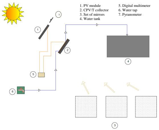
Figure 10. Schematic diagram of the experimental test setup
