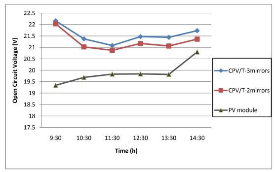
Figure 21. Variation of open circuit voltage versus time during the day of test
