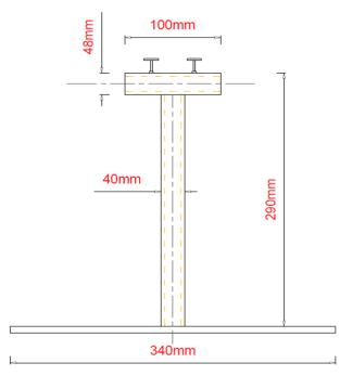
Figure 6. The metal pipe attached on the PV module and the PV/T collector
