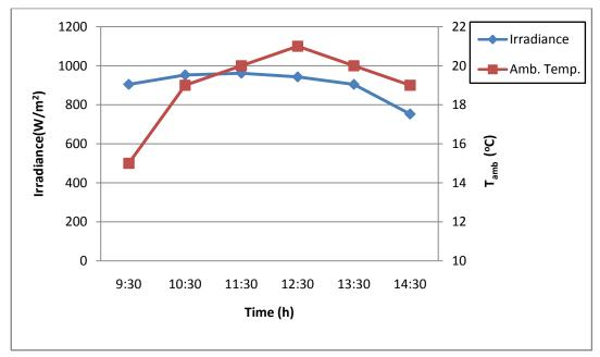
Figure 19. Variation of ambient temperature and solar irradiance during the test day
