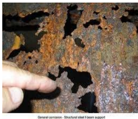
Figure 1.2: General attack corrosion [28]
