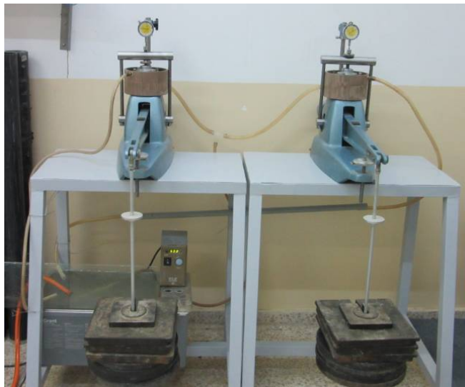
Figure 5.7. General view of temperature controlled oedometer system.
