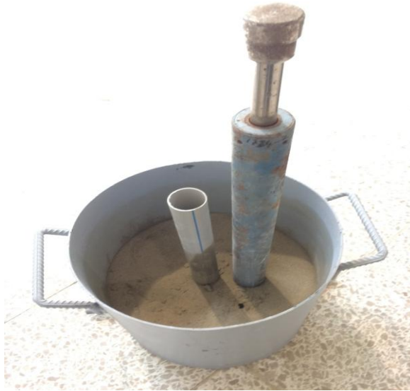
Figure 3.14: The compacted soil sample in the test tank
