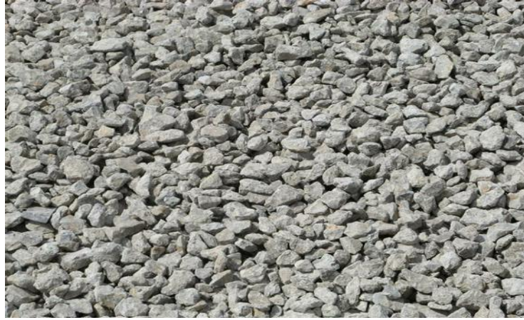
Figure 3.10: Sample of the crushed waste concrete
