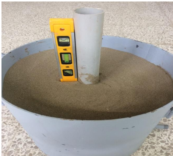
Figure 3.19 The vertical stone column
