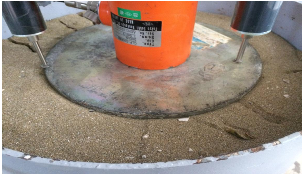
Figure 3.24: Sensitive settlement gauges fixed on the circular foundation
