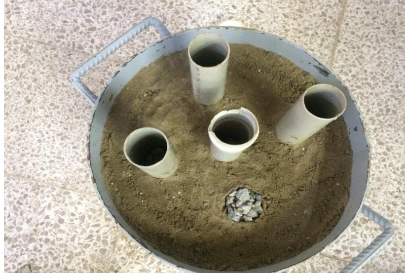
Figure 3.21: Extraction of stone columns
