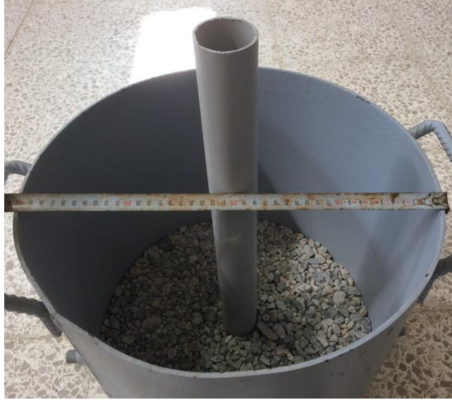
Figure 3.17: Installation of a single stone column into the test tank
