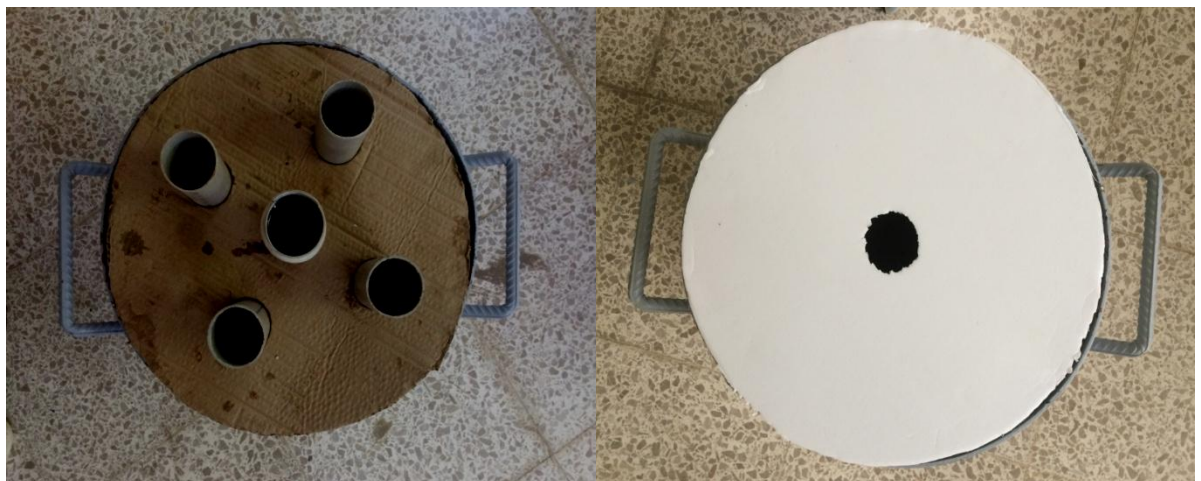
Figure 3.16: The pattern of single and group of stone columns
