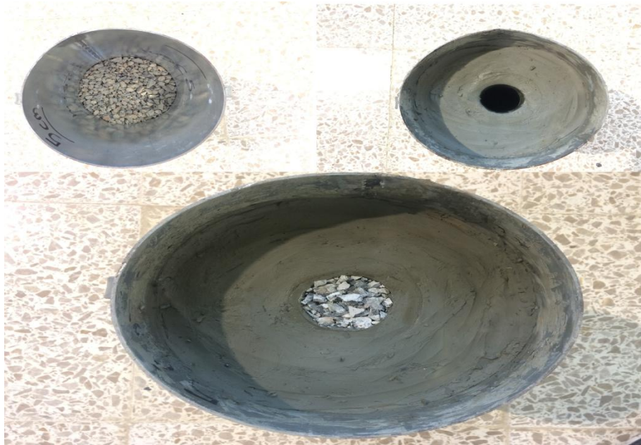
Figure 3.20 The stone columns and the soft clay in the test tank
