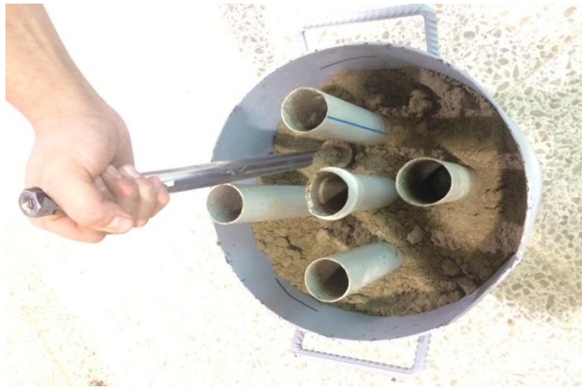
Figure 3.18: Installation process of single and group of columns in the test tank
