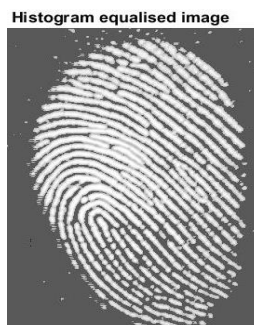
Figure 3.4: Histogram Equalization of Fingerprint Image (Define by Code Appendix A, at Line 24)
