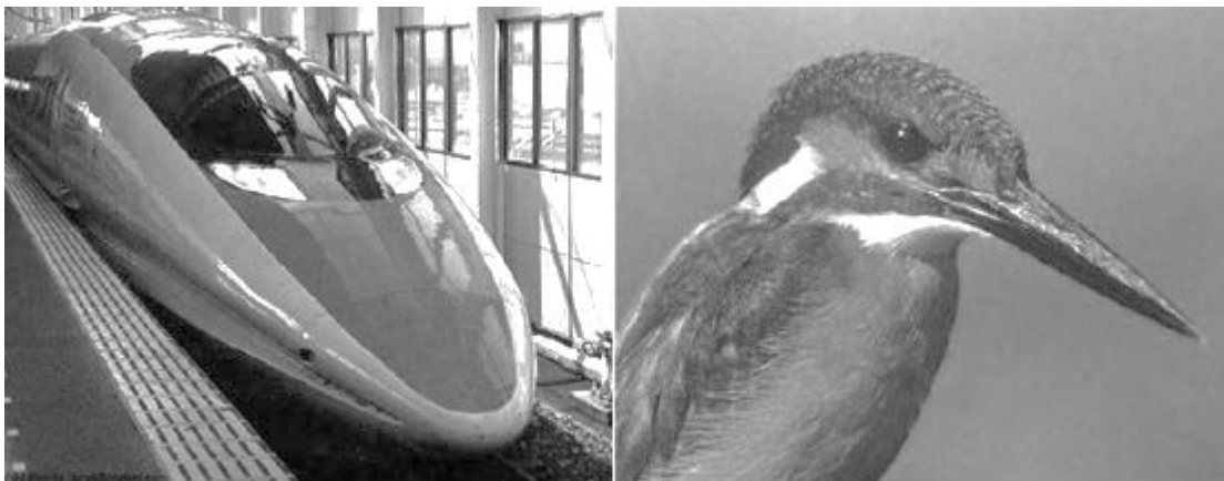
Figure 5. The Japanese bullet train modeled from kingfisher, which can dive into water for fishing without much of a splash (URL 24)
