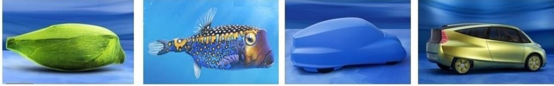
Figure 10. Daimler Chrysler bionic car that is inspired from boxfish and tree growth pattern (URL 17)
