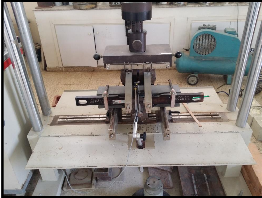
Figure 4.1: Flexural toughness test
