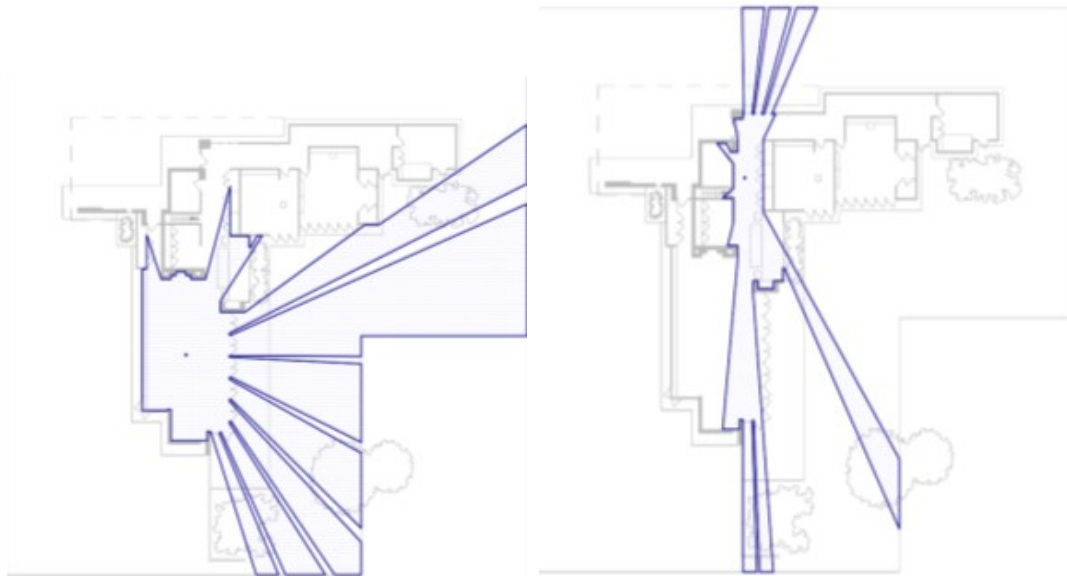
Figure 10: Representation of the isovists in an architectural plan (Frank Lloyd Wright's Jacobs House)
