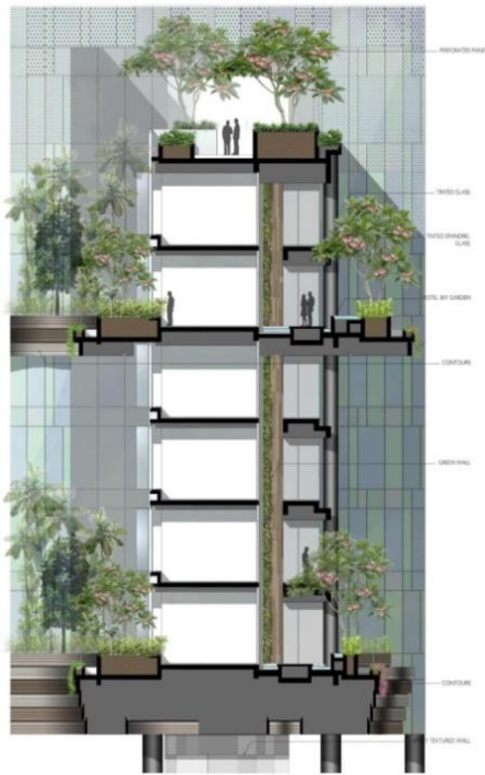
Figure 77: Cross section detail of integrated vertical vegetation and vertical green systems (Patrick Bingham-Hall, 2014)
