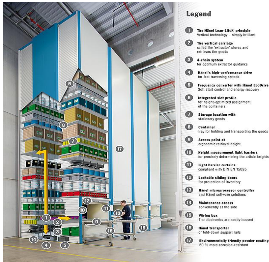
Figure 2.3: Vertical lift storage at Hanel Storage Systems [67].
