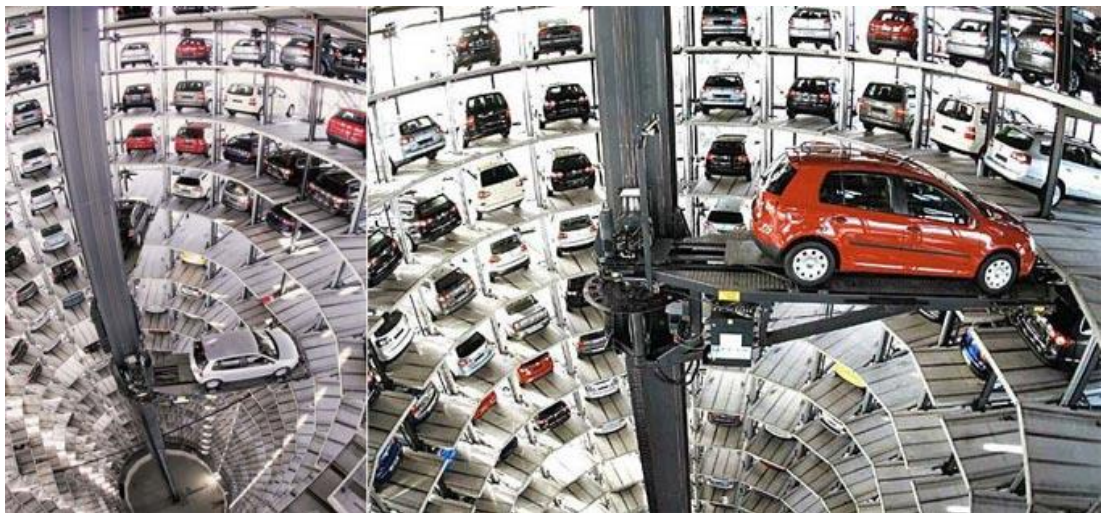
Figure 1.4: Circular Type ASRS of Volkswagen Company [65, 66]
