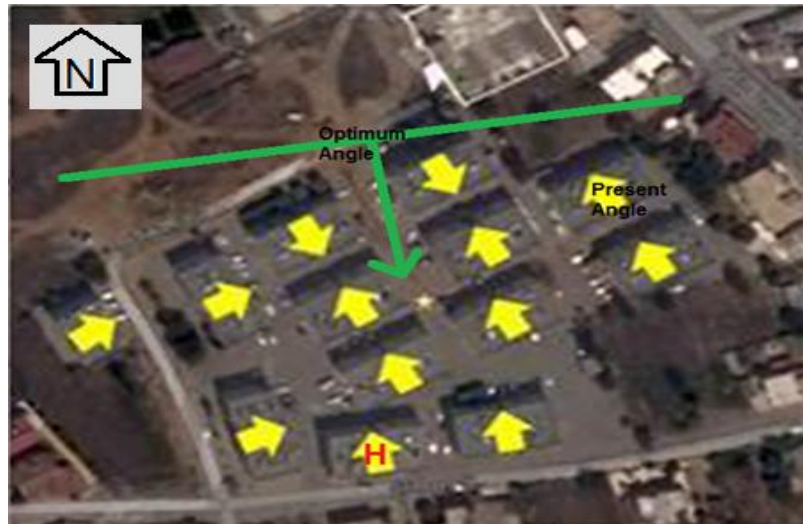
Figure 36. The Azimuth Angle of Haci Ali Blocks on Site (Case I)
