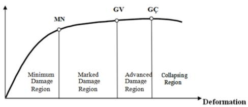
Figure 2.2. Member damage levels and member performance regions on capacity curve [9].
