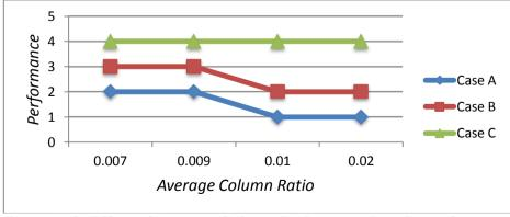
Figure 5.10. Effect of Average Column Ratio on earthquake performance 81
