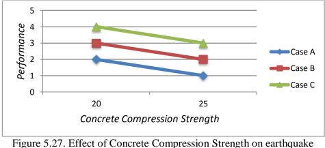
gure 5.27. Effect of Concrete Compression Strength on earthquake performance
