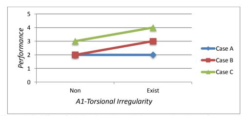
Figure 5.18. Effect of A1-Torsional Irregularity on earthquake performance
