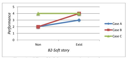
Figure 5.6. Effect of Soft Storey on earthquake performance
