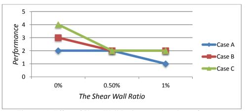
Figure 5.1. Effect of Shear Wall Ratio on earthquake performance
