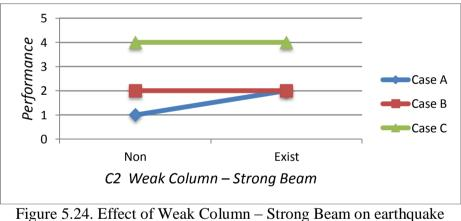
figure 5.24. Effect of Weak Column – Strong Beam on earthquake performance
