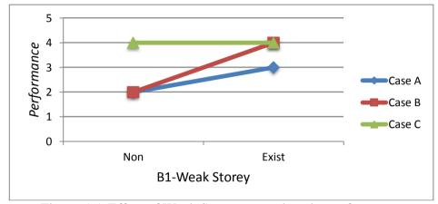
Figure 5.5. Effect of Weak Storey on earthquake performance
