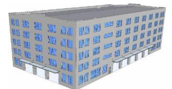
Figure 4.6. Illustration of a building with a soft ground story due to large openings and narrow piers.
