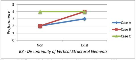
Figure 5.7. Effect of B3 - Discontinuity of Vertical Structural Elements on earthquake performance
