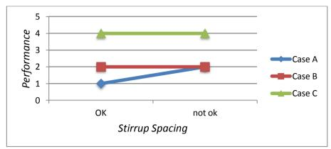
Figure 5.25. Effect of Stirrup Spacing on earthquake performance
