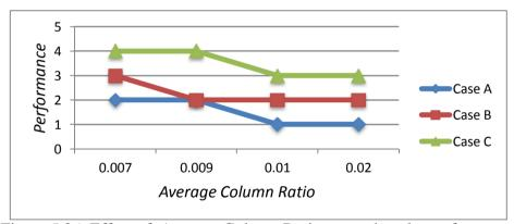
Figure 5.26. Effect of Average Column Ratio on earthquake performance
