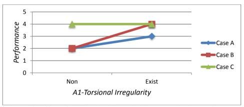
Figure 5.2. Effect of A1-Torsional Irregularity on earthquake performance
