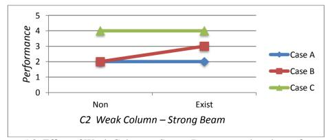
Figure 5.8. Effect of Weak Column – Strong Beam on earthquake performance
