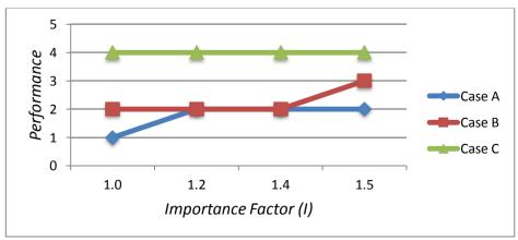
Figure 5.16. Effect of Importance Factor (I) on earthquake performance
