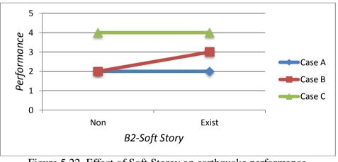
Figure 5.22. Effect of Soft Storey on earthquake performance
