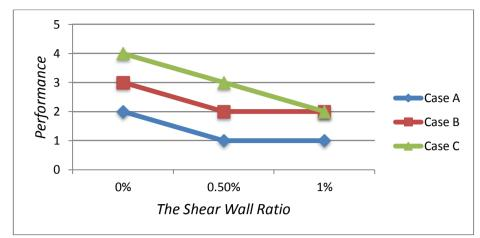
Figure 5.17. Effect of Shear Wall Ratio on earthquake performance
