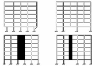
Figure 4.8. Type B3- Discontinuities of Vertical Structural Elements [9].
