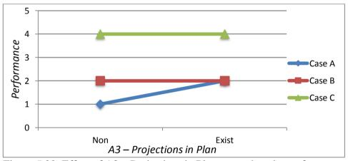
Figure 5.20. Effect of A3 – Projections in Plan on earthquake performance
