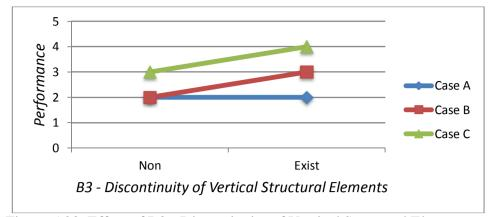
Figure 5.23. Effect of B3 - Discontinuity of Vertical Structural Elements on earthquake performance
