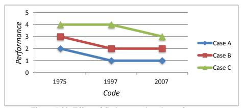
Figure 5.30. Effect of Code on earthquake performance
