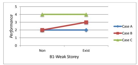
Figure 5.21. Effect of Weak Storey on earthquake performance
