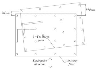
Figure 4.2. Type A1- Torsional Irregularity [9].
