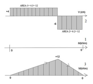
Figure 9.33. Steps of drawing an M diagram
