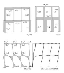
Figure 9.50. N, V, M diagrams and the deflected shape of the frame
