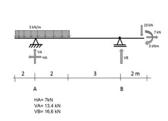
Figure 9.36. A system to draw N,V,M diagrams and deflected shape
