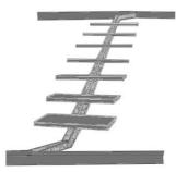
Figure 9.15. Transfer of the weight of the flight to the frame through beams
