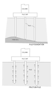
Figure 9.24. Pile foundations
