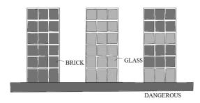
Figure 9.64. Acceptable and unacceptable arrangements of rigid partition walls and windows within frame systems
