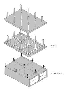
Figure 9.23. Various applications of raft foundation
