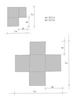
Figure 9.60. Avoiding deep recesses with the help of expansion joints
