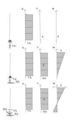
Figure 9.40. Types of columns in determinate systems
