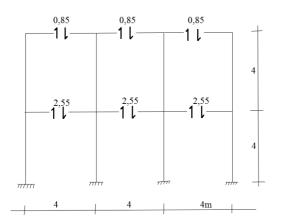
Figure 9.47. Finding shear in beams
