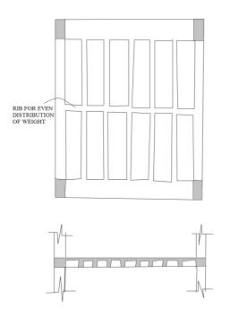
Figure 9.9. Structural plan and sections of a ribbed slab
