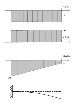
Figure 9.39. N,V,M diagrams and deflected shape of the system in Figure 9.38
