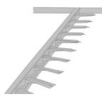
Figure 9.17. Cantilevering steps
