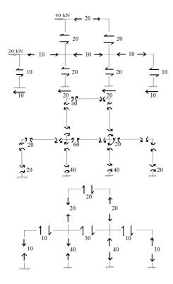
Figure 9.52. Finding internal forces in the elements of the frame
