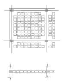
Figure 9.11. Structural plan and section of a waffled slab
