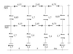
Figure 9.49. Finding axial force in beams
