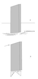
Figure 9.27. a. Minimum dimensions of reinforced concrete shear walls b. Transfer of horizontal load by reinforced concrete shear walls
