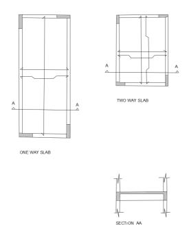
Figure 9.7. Structural plan (with reinforcement) and section of one way and two way slabs
