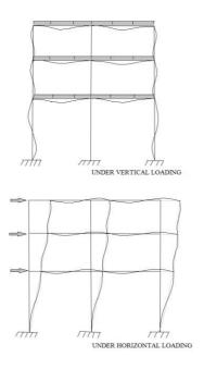
Figure 9.2. Deformation of frames under vertical and horizontal loads
