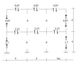
Figure 9.48. Finding axial force in columns
