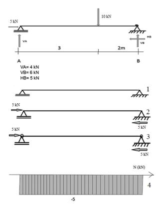
Figure 9.31. The four steps of drawing an N diagram
