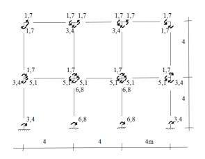
Figure 9.46. Finding moments in columns and beams
