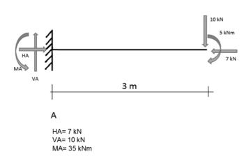
Figure 9.38. Another system to draw N,V,M diagrams and deflected shape
