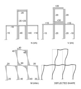
Figure 9.53. N, V, M diagrams and the deflected shape of the frame
