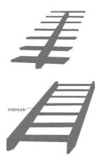
Figure 9.14. Structure of a flight
