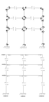
Figure 9.3. Axial force and shear force in the elements of frames
