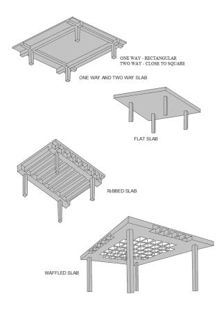
Figure 9.6. Reinforced concrete slab types
