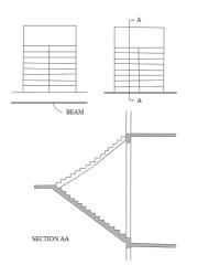
Figure 9.18. Whole stair-case as a cantilever
