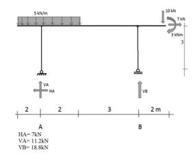
Figure 9.43. Another system with columns to draw N,V,M diagrams and deflected shape Figure 9.44 shows the N,V,M diagrams and deflected shape of the system shown in Figure 9.43.
