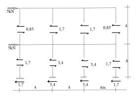
Figure 9.45. Finding shear in columns
