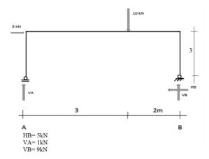
Figure 9.41. A system with columns to draw N,V,M diagrams and deflected shape
