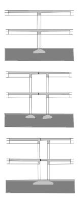
Figure 9.26. Different applications of expansion joints
