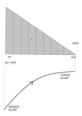
Figure 9.35. Drawing parabolic curves in the M diagram
