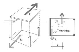
Figure 9.62. Earthquake force F and resistance of structure R
