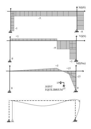
Figure 9.42. N,V,M diagrams and deflected shape of the system in Figure 9.41
