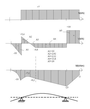
Figure 9.37. N,V,M diagrams and deflected shape of the system in Figure 9.36 Example 9.2. Draw the N,V,M diagrams and the deflected shape of the system shown in Figure 9.38.
