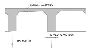
Figure 9.10. Dimensions of ribs
