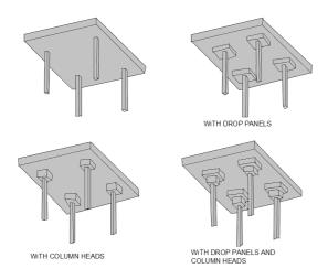
Figure 9.8. Different applications of flat slab
