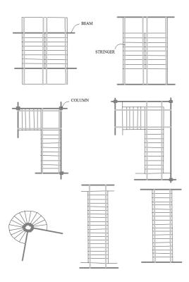
Figure 9.16. Use of beams to carry flights and landings in different arrangements
