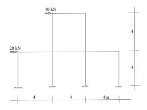
Figure 9.51. A frame to draw N,V,M diagrams and deflected shape
