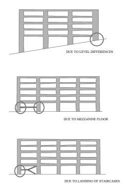
Figure 9.67. Some other causes of short column problems
