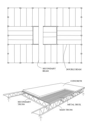
Figure 9.13. Use of secondary steel beams and trusses
