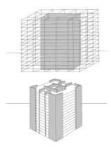
Figure 9.30. Distribution of shear walls within the structure
