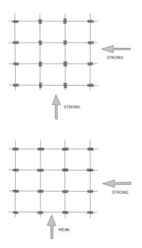
Figure 9.5. Directions of the columns in plan
