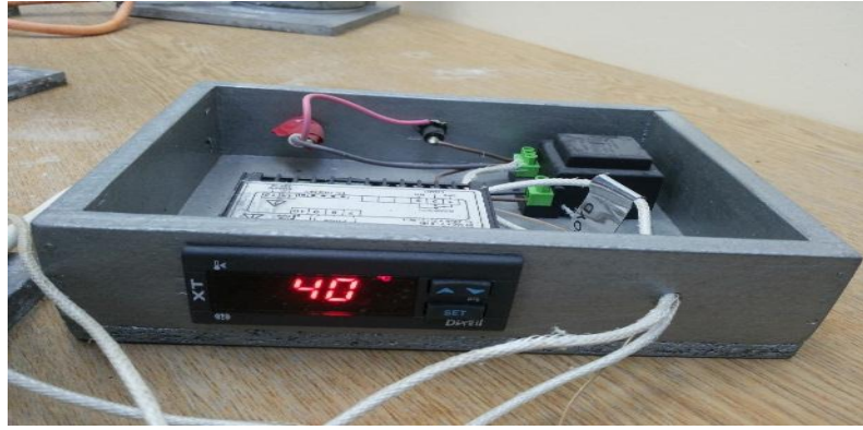
Figure 3.4: The Temperature Controller Used for Drying Stage
