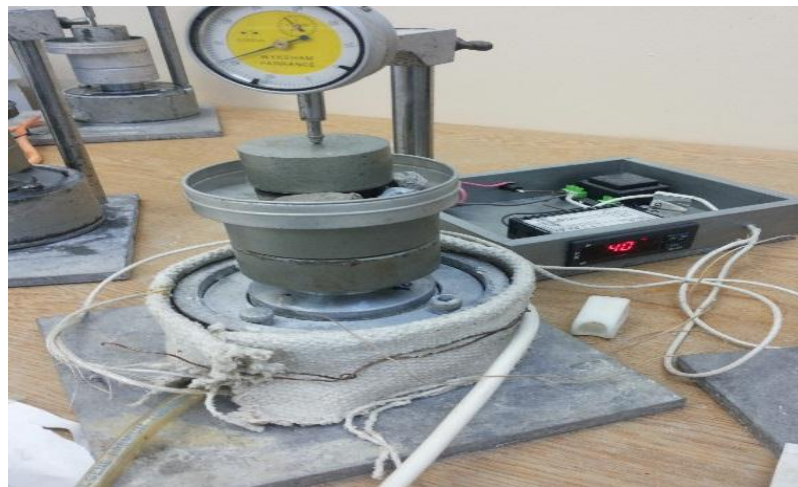
Figure 3.5: The Flexible Heater and the Test Set up Used for Drying Stage
