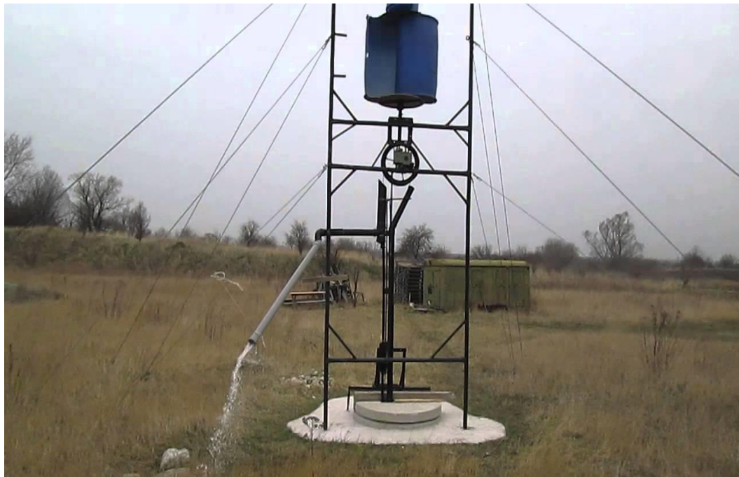
Figure 6 : Savonius wind turbine for pumping water
