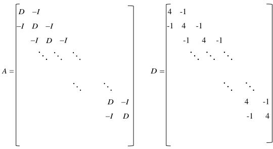
Figure 2.4: Structure of the Coefficient Matrix Using 5-point Scheme and Lexicographical Ordering
