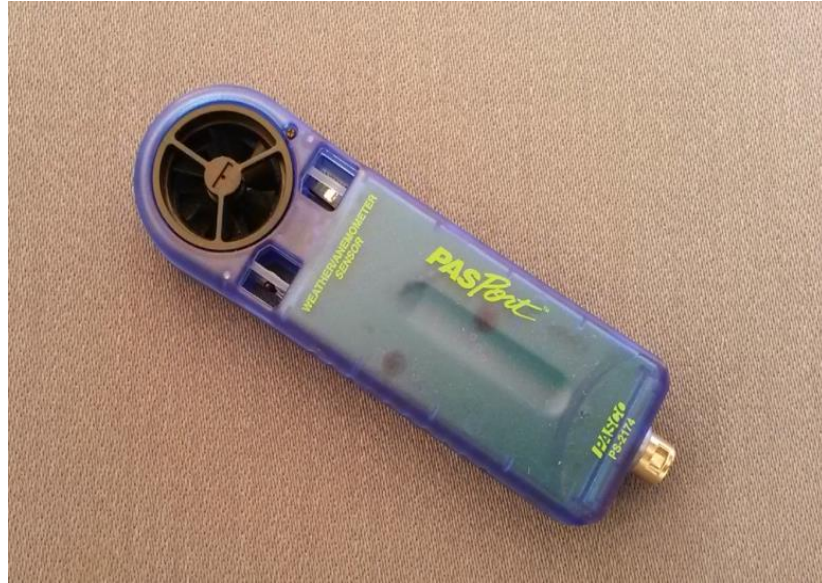
Figure 4.5: Photograph of Anemometer sensor.
