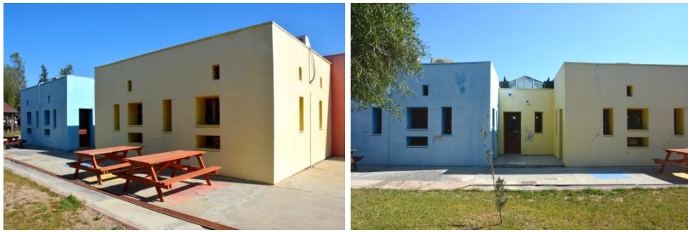
Figure 60: Modular windows in child-scaled height, upper windows for natural ventilation and extra access to the balcony from classroom - S.O.S Kindergarten (Direct Observation on 22/02/2016)
