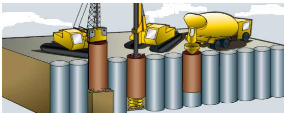
Figure 2.16: Procedure of sequential bored piles wall construction [11]
