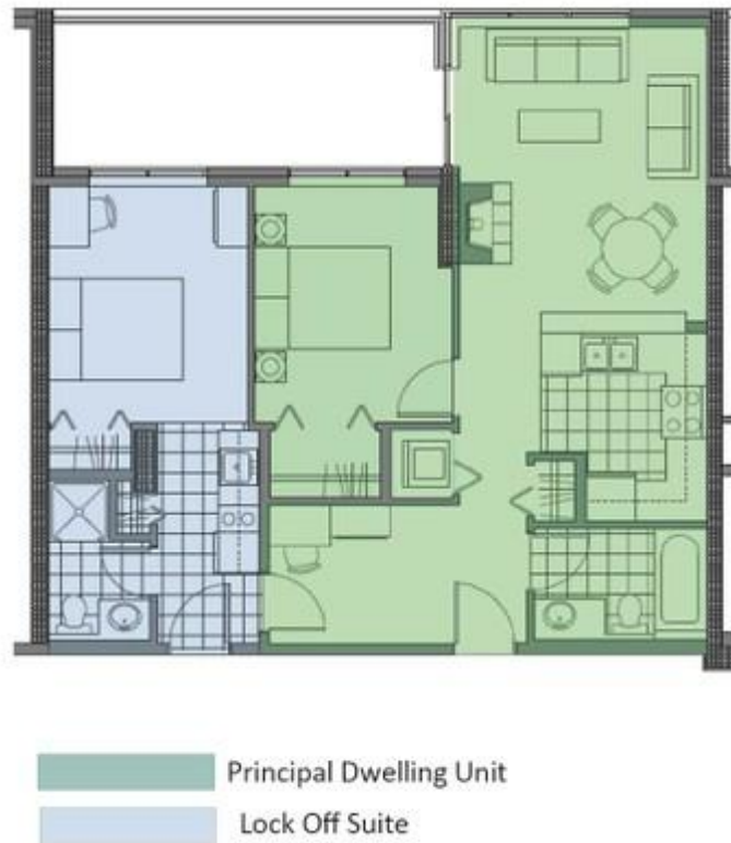
Figure 15: Example of lock-off suit attached to a dwelling unit. (URL:9)
