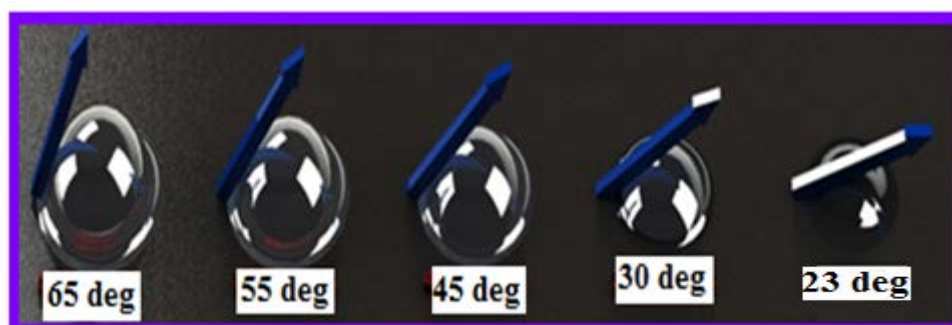
Figure 5.23: Wettability of scaffold nanocomposite containing various amounts of MNPs
