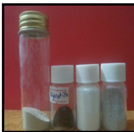
Figure 5.6: Nanocomposite and magnetite powders prepared by HEBM and sol-gel technique
