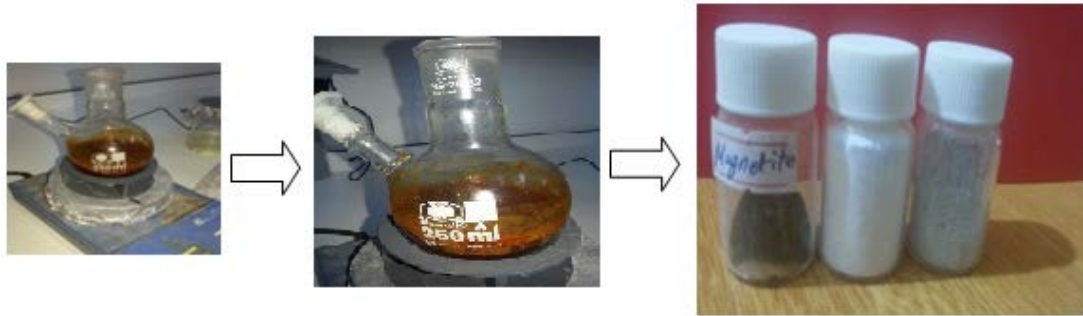
Figure 3.4: Prepared magnetite powders by sol-gel method
