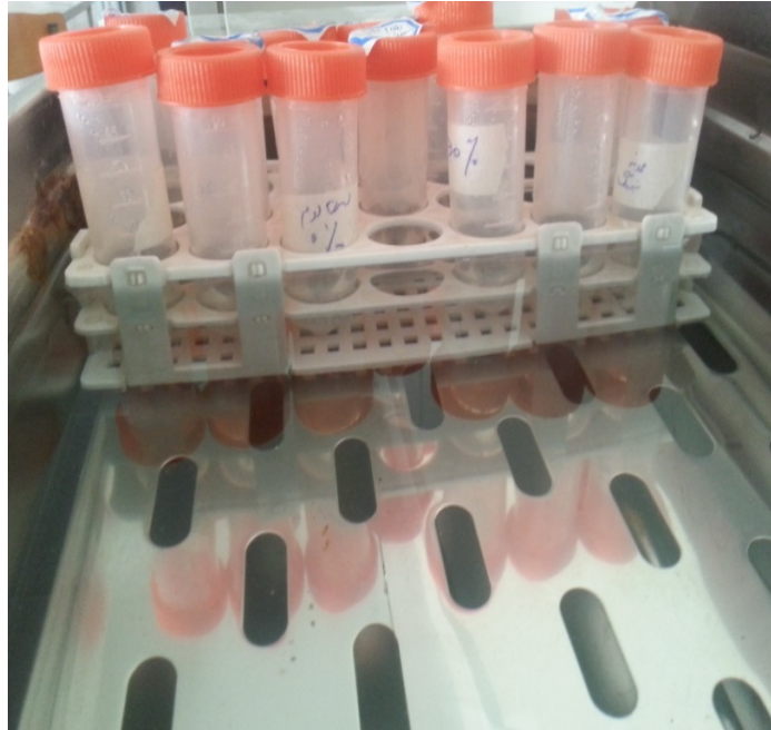
Figure 3.8: The falcon tubes and samples soaked in the SBF and PBS solution for 4 weeks in the bain marie bath (similar to human's body condition)
