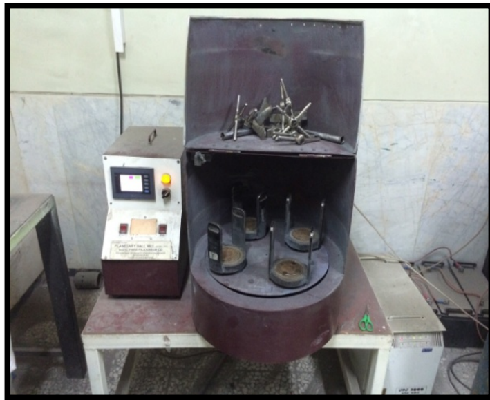
Figure 3.2: Schematic of planetary HEBM technique to synthesize based materials
