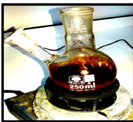
Figure 5.8: Preparation of magnetite powders by sol-gel technique
