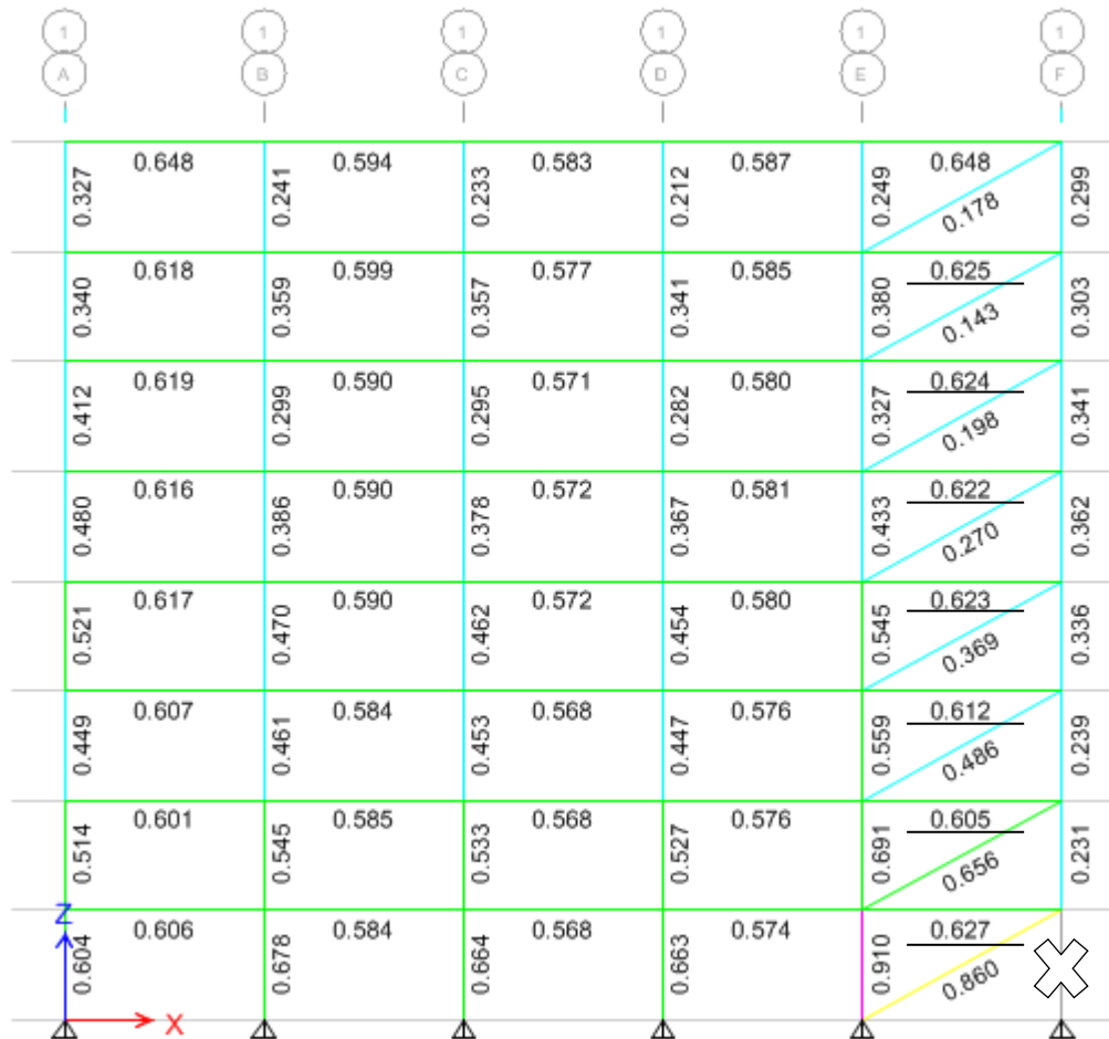
Figure 4.30: DCRs after rehabilitating RB-I Case 4 - column is removed from the corner of the building.
