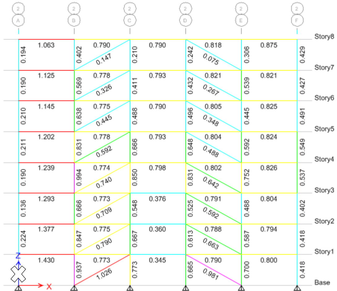
Figure 4.20: DCRs IR4F-I Case 1 - column is removed from the short side of the building.
