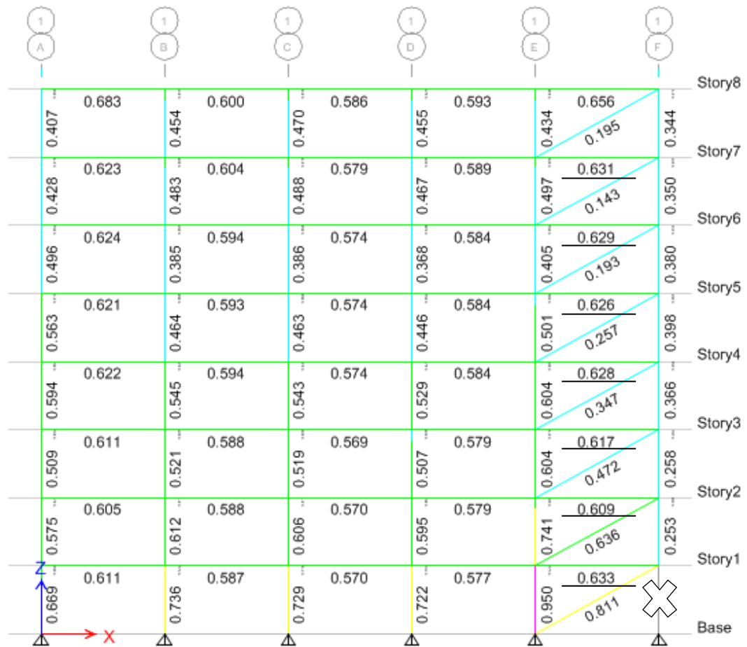
Figure 4.33: DCRs after rehabilitating RB-T Case 4 - column is removed from the corner of the building.
