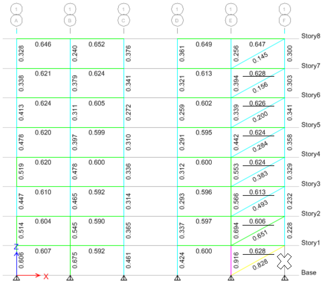
Figure 4.36: DCRs after rehabilitating IR8F-I Case 4 – column is removed from the side corner of the building.
