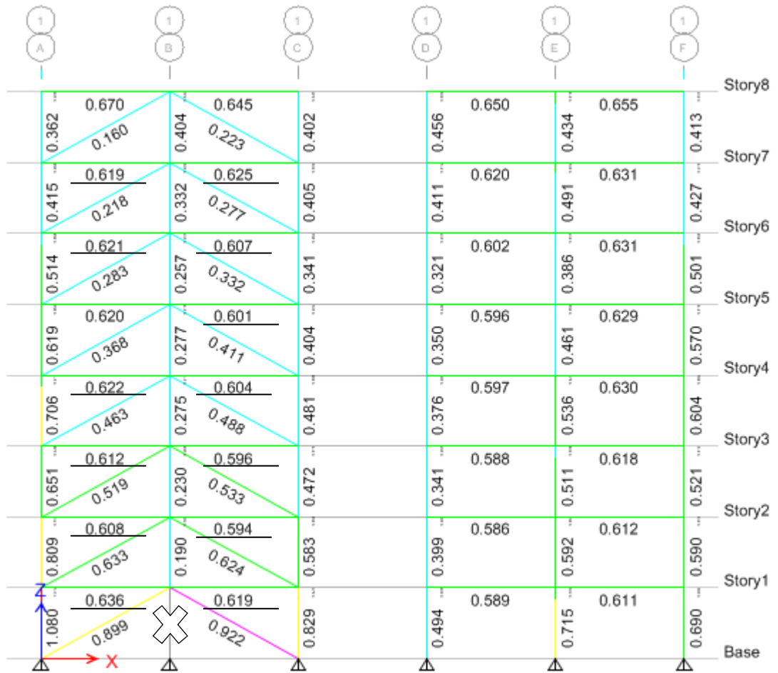
Figure 4.37: DCRs after rehabilitating IR8F-T Case 2 – column is removed from the long side (Gr1B) of the building.
