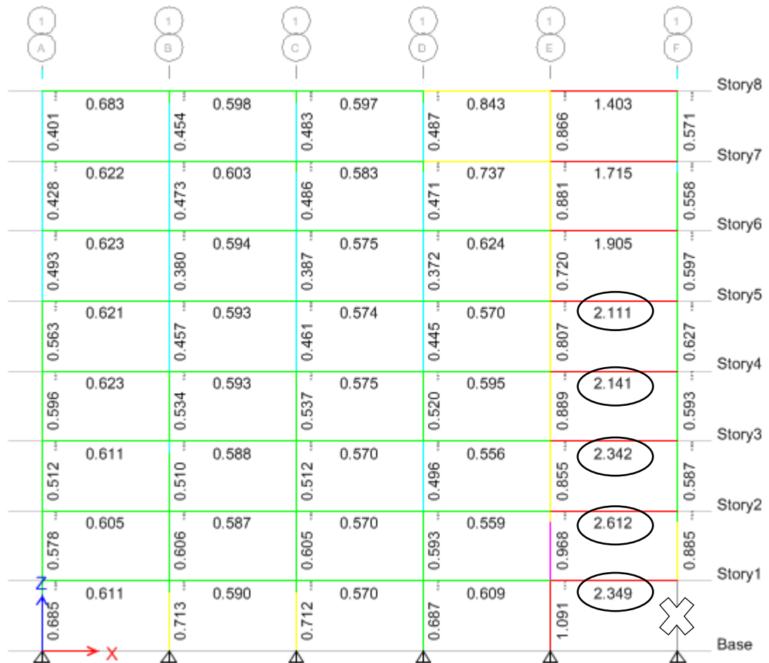
Figure 4.9: DCRs RB-T Case 4 - column is removed from the corner of the building.
