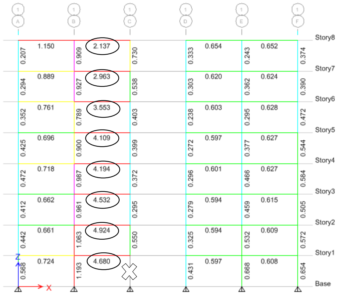
Figure 4.13: DCRs IR8F-I Case 3 - column is removed from the long side (Gr1C) of the building.
