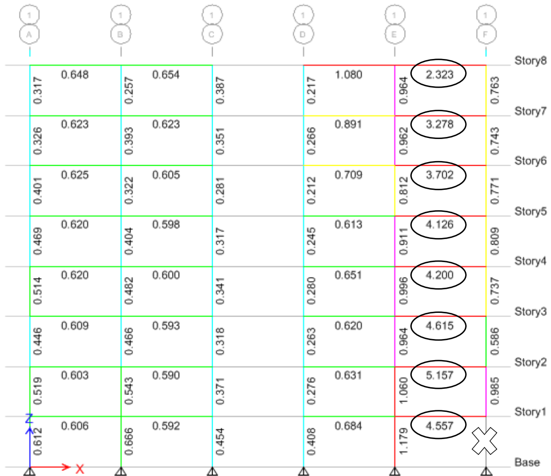
Figure 4.14: DCRs IR8F-I Case 4 - column is removed from the corner of the building.
