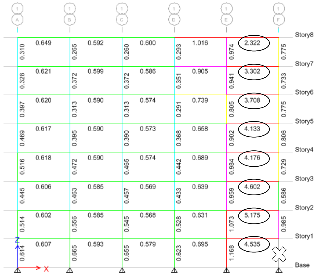
Figure 4.5: DCRs for RB-I Case 4 - column is removed from the corner of the building.
