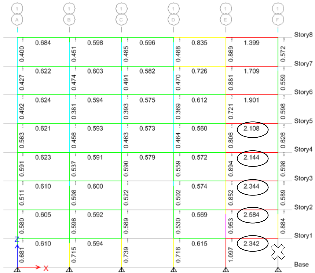
Figure 4.27: DCRs IR4F-T Case 4 - column is removed from the corner of the building.
