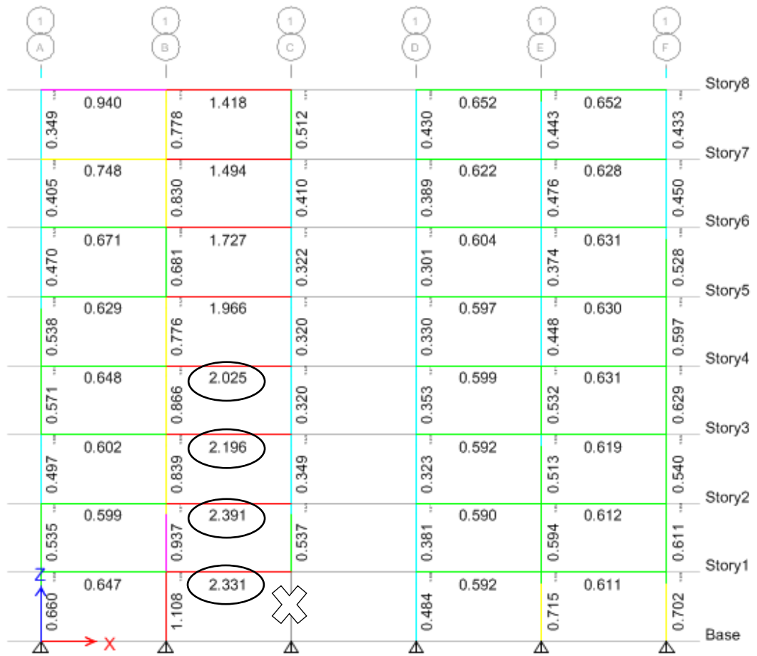
Figure 4.17: DCRs IR8F-T Case 3 - column is removed from the long side (Gr1C) of the building.
