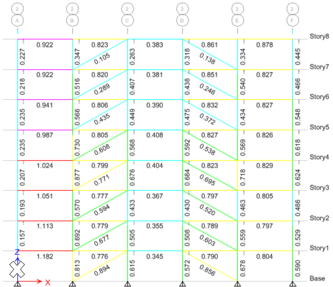
Figure 4.15: DCRs IR8F-T Case 1 - column is removed from the short side of the building.
