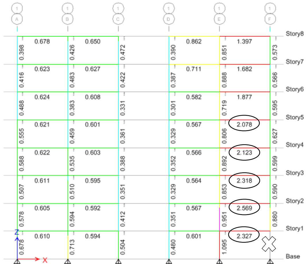
Figure 4.18: DCRs IR8F-T Case 4 - column is removed from the corner of the building.
