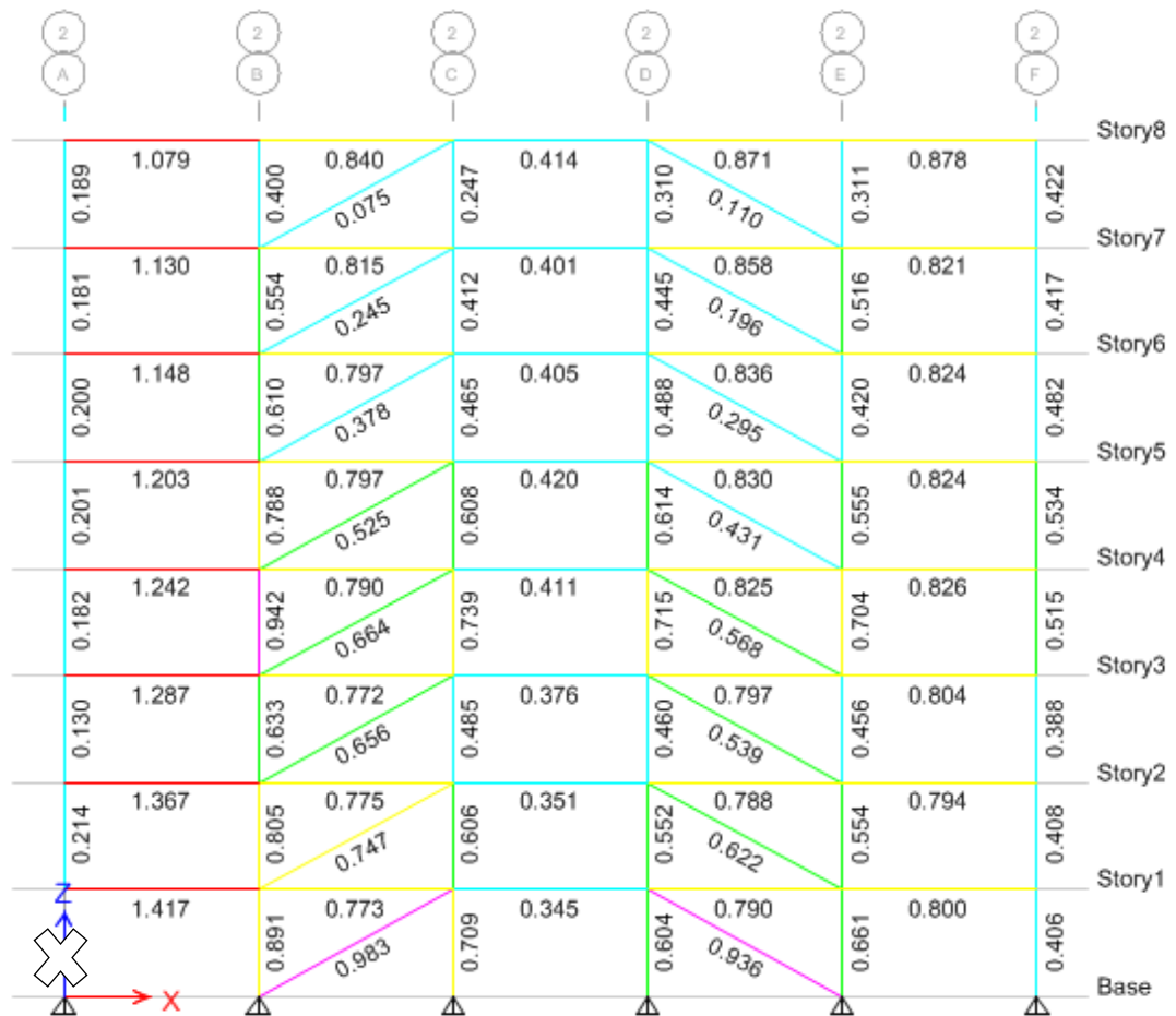
Figure 4.11: DCRs IR8F-I Case 1 - column is removed from the short side of the building.
