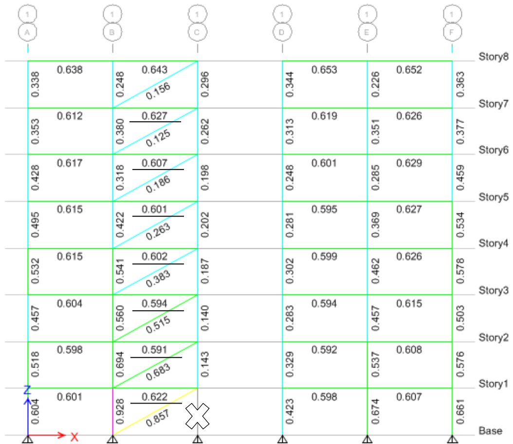
Figure 4.35: DCRs after rehabilitating IR8F-I Case 3 – column is removed from the long side (Gr1C) of the building.
