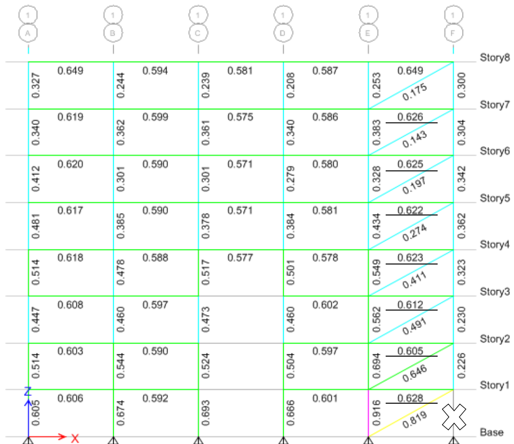
Figure 4.42: DCRs after rehabilitating IR4F-I Case 4 – column is removed from the corner of the building.
