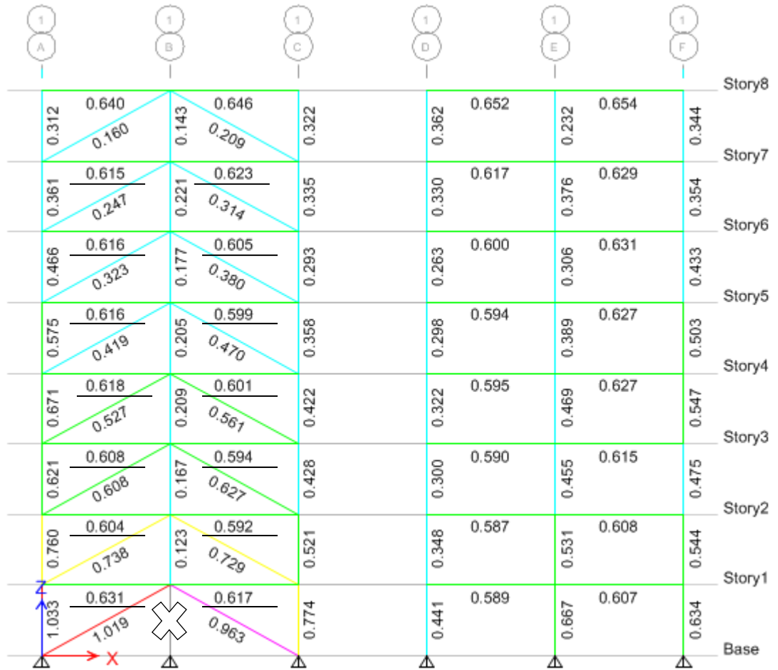
Figure 4.34: DCRs after rehabilitating IR8F-I Case 2 – column is removed from the long side (Gr1B) of the building.
