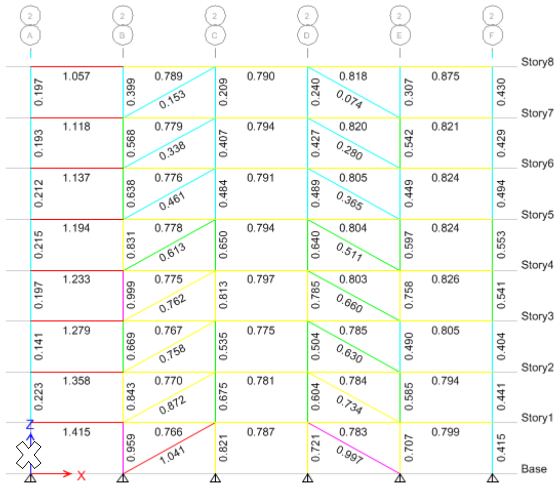
Figure 4.2: DCRs for RB-I Case 1 - column is removed from the short side of the building.
