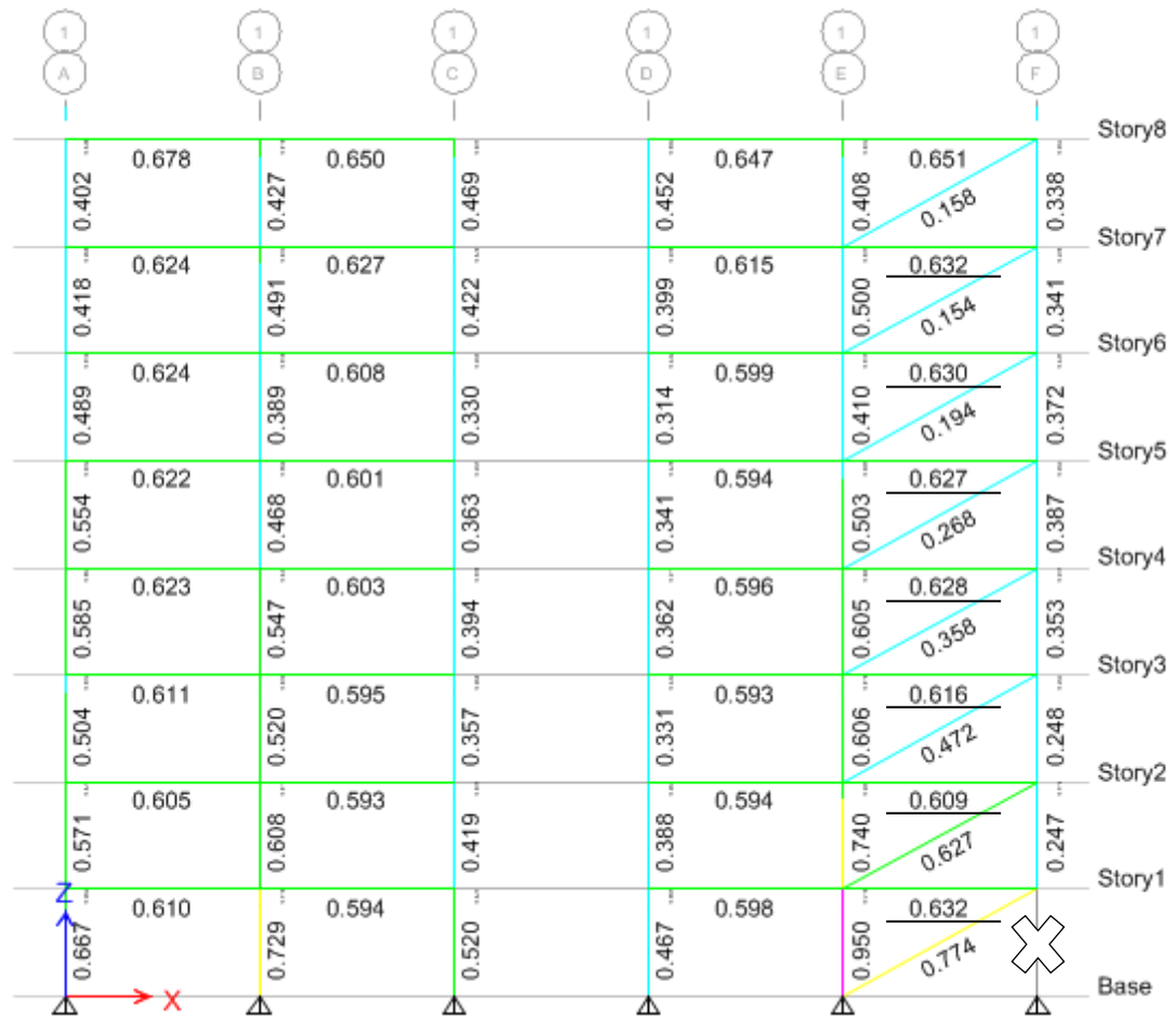
Figure 4.39: DCRs after rehabilitating IR8F-T Case 4 – column is removed from the corner of the building.
