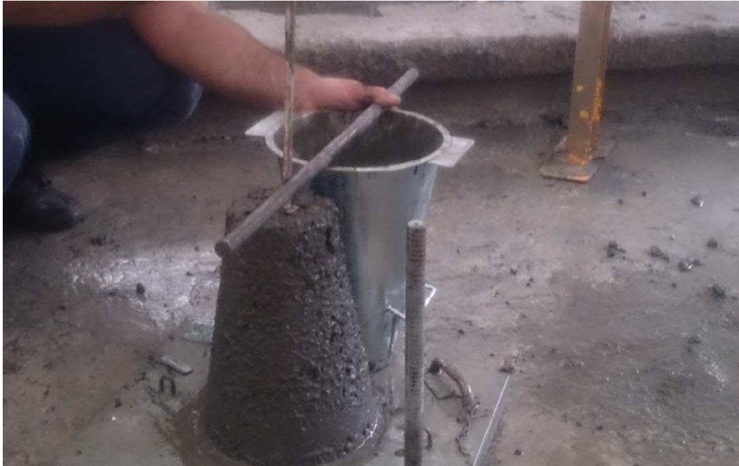
Figure 4: Measurement of Slump Value – Slump Test
