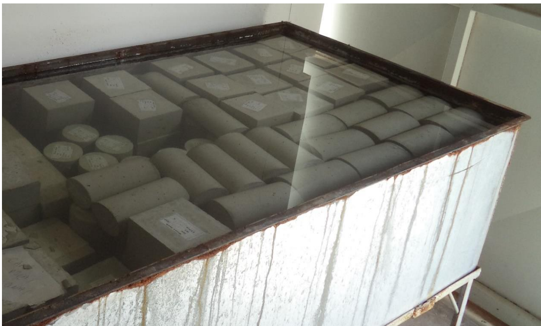
Figure 6: Standard Curing of Specimens – Curing Tank
