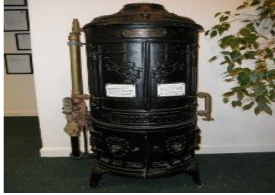
Figure 3: Instantaneous Water Heater of 1904 as illustrated in Ref. [10]
