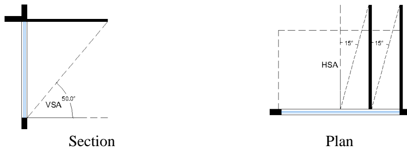
Figure 51: West orientation solar shading element 50o degree angle (VSA) for overhangs and 15 degree angle (HSA) for vertical fins. (Drawn by author)
