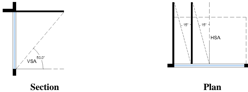
Figure 49: East orientation solar shading element 50o degree angle (VSA) for overhangs and 15 degree angle (HSA) for vertical fins (Drawn by author).
