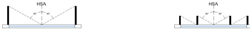
Figure 53: North orientation solar shading element 60° degree angle (HSA) for vertical fins. (Drawn by author).
