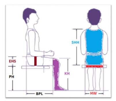
Figure 5.1: the six body measurements for seat and table design
