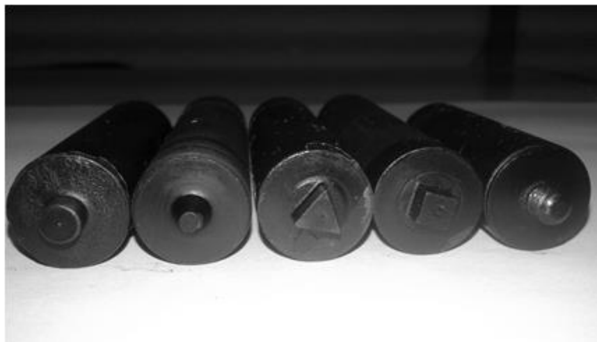
Figure 20. FSP tool pin profiles: (a) straight cylindrical, (b) taper cylindrical, (c) threaded cylindrical, (d) triangular, and (e) square
