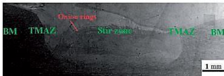
Figure 23. The typical cross-sectional macrostructure of the processed
