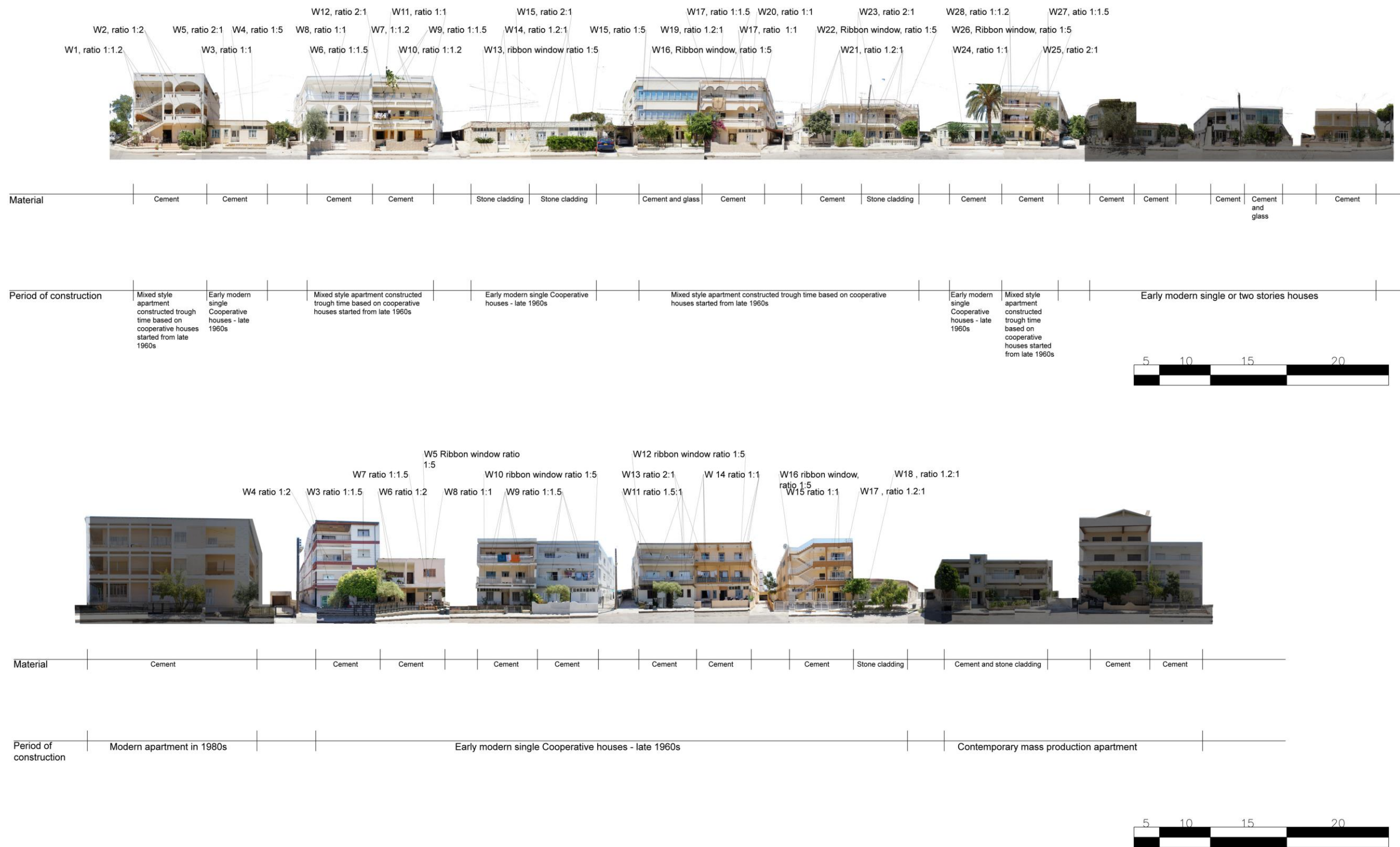
Figure 38. Façade characteristics of early modern cooperative houses and mixed style apartments constructed through time based on cooperative houses in Samsun street of Baykal region (Author, 2016)
