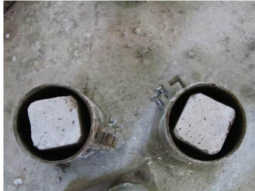
Figure 3.16: Shape-modification of square samples by using circular molds
