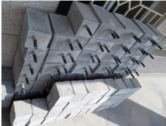
Figure 3.15: Storing the specimens in the laboratory before CFRP wrapping
