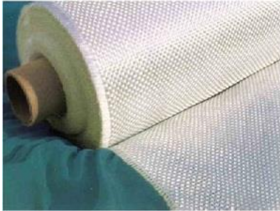
Figure 2.8: Glass Fiber Reinforce Polymer (GFRP) sheet [62]
