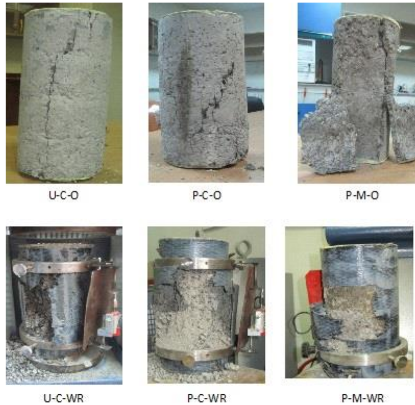
Figure 4.2: Failure of circular and modified specimens
