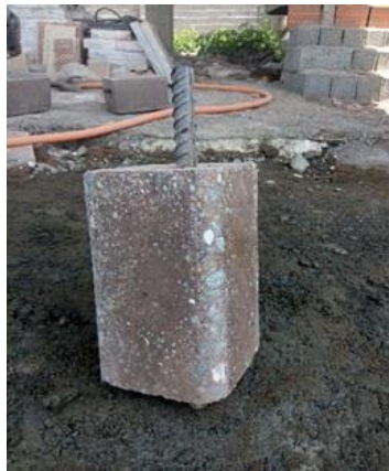
Figure 3.18: Sample prepared according to standard before installation
