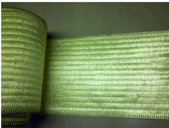
Figure 2.9: Aramid Fiber Reinforce Polymer (AFRP) sheet [62]
