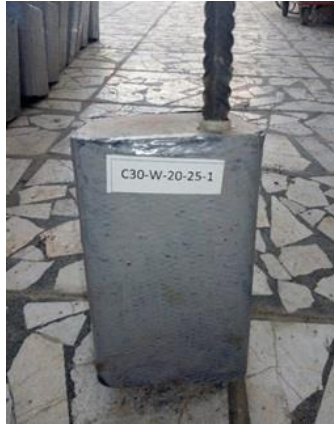
Figure 3.19: CFRP applied on specimens
