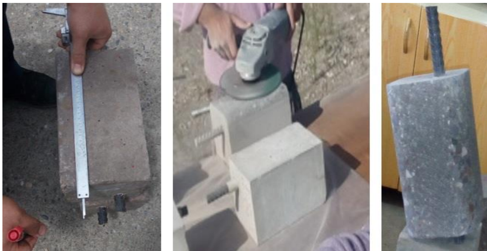
Figure 3.17: Corner rounded specimens to 20 mm radius in cross sections
