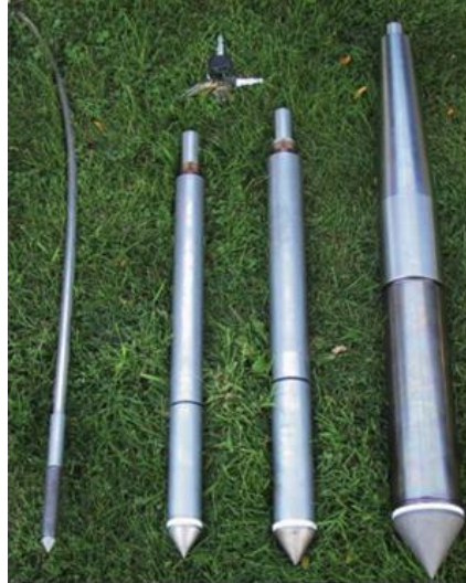
Figure 4.1: Range of CPT Probes (from left: 2 cm 2 , 10 cm 2 , 15 cm 2 , 40 cm 2 )
