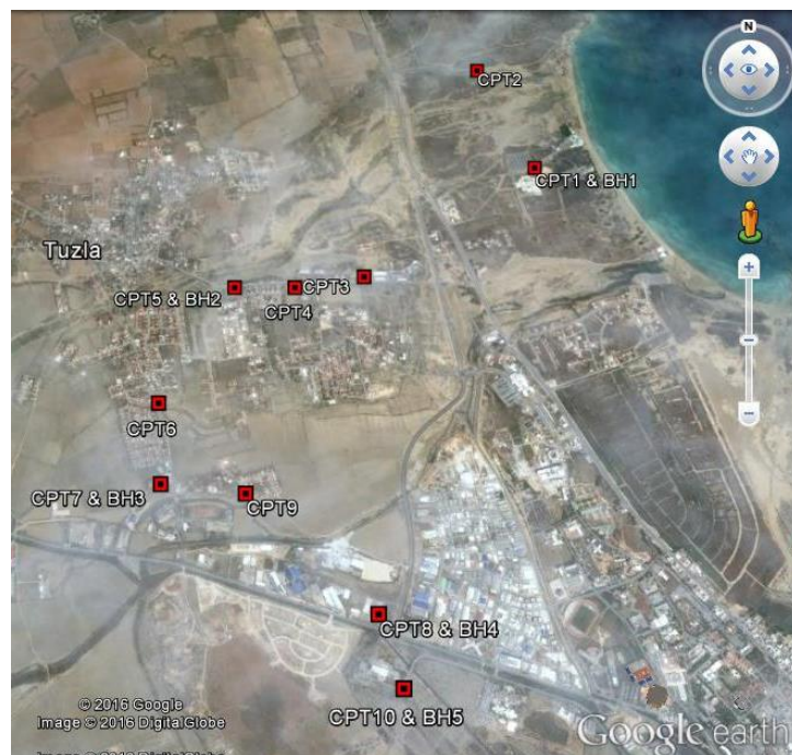
Figure 5.1: CPT Locations in the Study Area (Google Earth Image of Tuzla, 35° 09'15" N 33°52' 58.91"), (Erhan, 2009).
