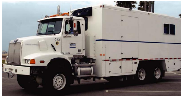
Figure 4.2: The CPT Truck used in the General Study.
