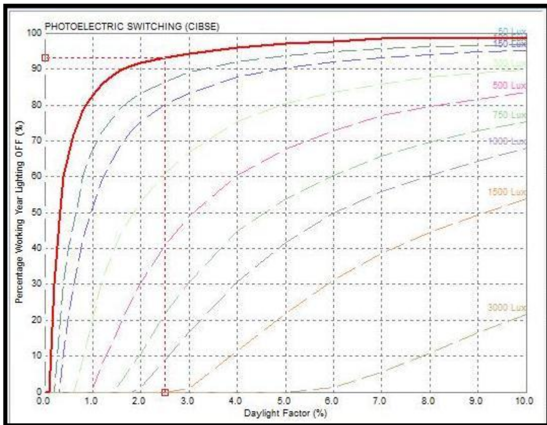
Figure 20: Photoelectric sensing effect chart (by author)
