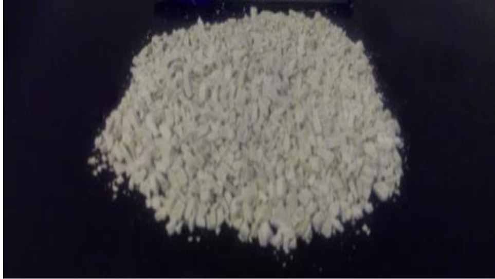
Figure 3.3: PVC Waste Plastics Crushed To 10 mm Maximum Size
