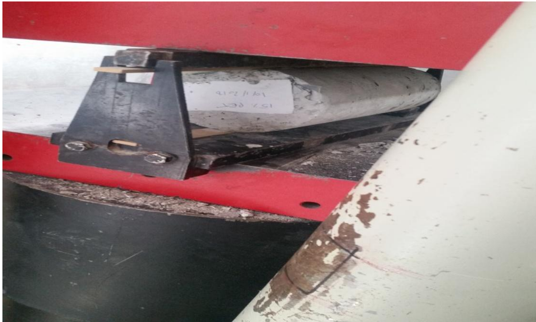
Figure 3.11: Splitting Tensile Testing Apparatus
