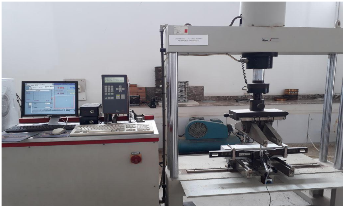
Figure 3.15: Flexural Toughness Test Arrangement with Yoke
