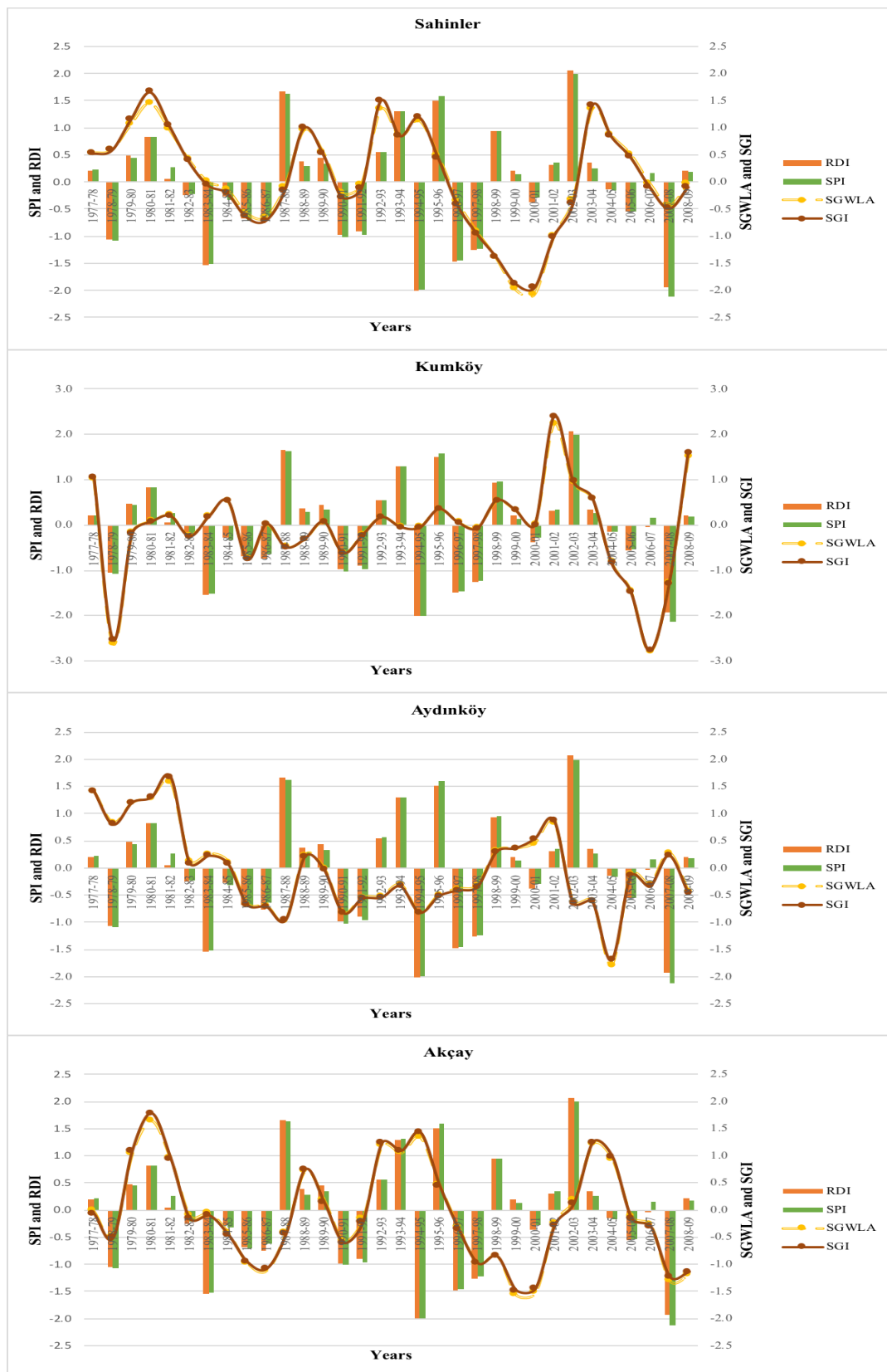
Figure 4.3(continued): Spatio-temporal comparison of SGWLA & SGI and SPI & RDI in different locations of Güzelyurt/Morphou Aquifer.
