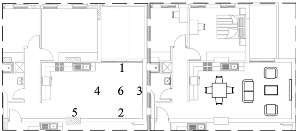
Figure 36: Furniture Placement by Contractor Firm (Alasya Park Flat Type 3)
