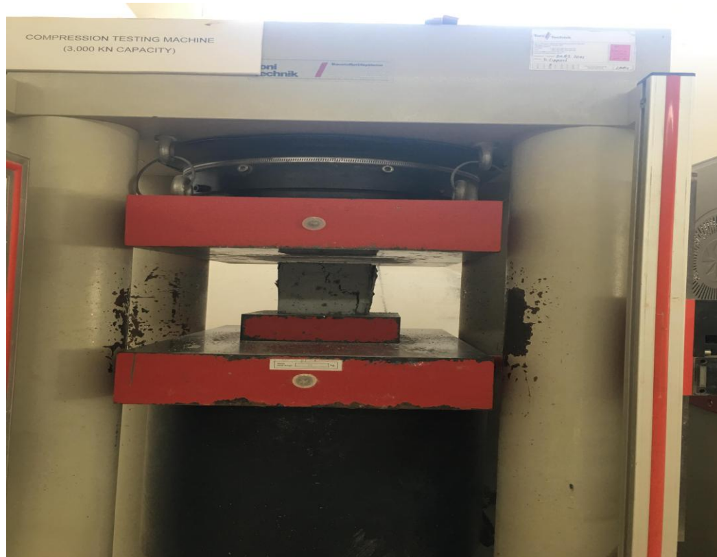
Figure 7: Compressive Strength Testing Equipment
