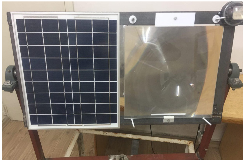
Figure 17: The plate with Fresnel lens and PV panel
