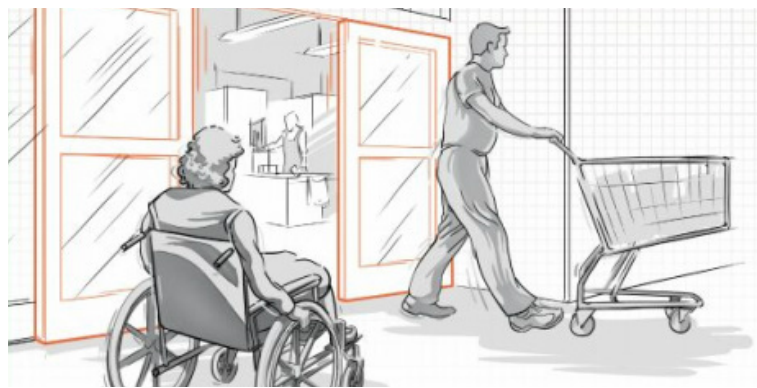
Figure 27: Sliding doors at the entrances that are convenient for all users.
