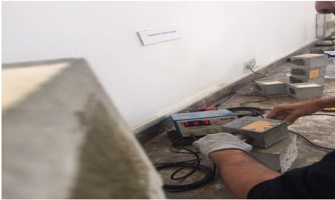
Figure 13: UPV test on the cubic sample
