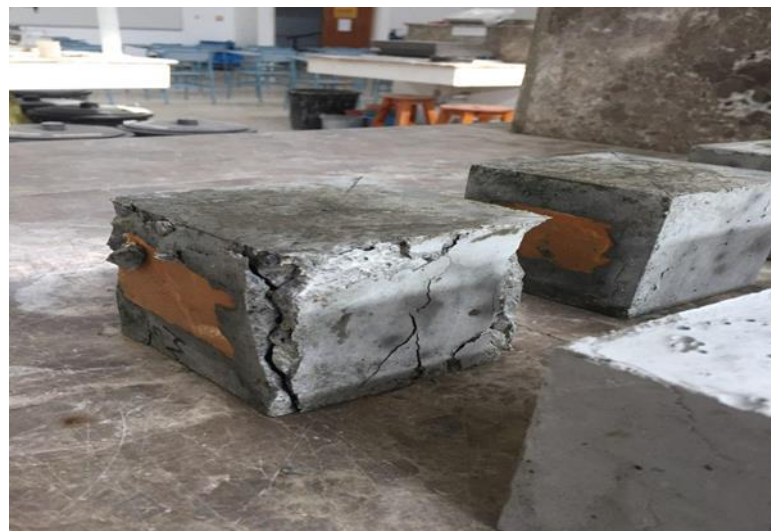
Figure 7: Specimen after compressive strength test
