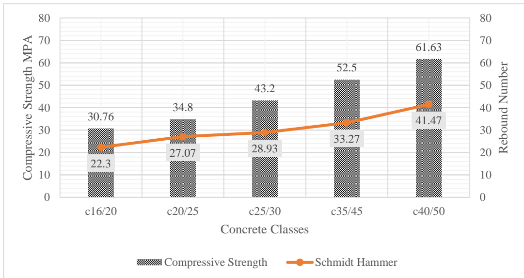
Figure 29: Schmidt hammer versus compressive strength results at 28 days age for concretes designed by ACI method for water tank curing regime
