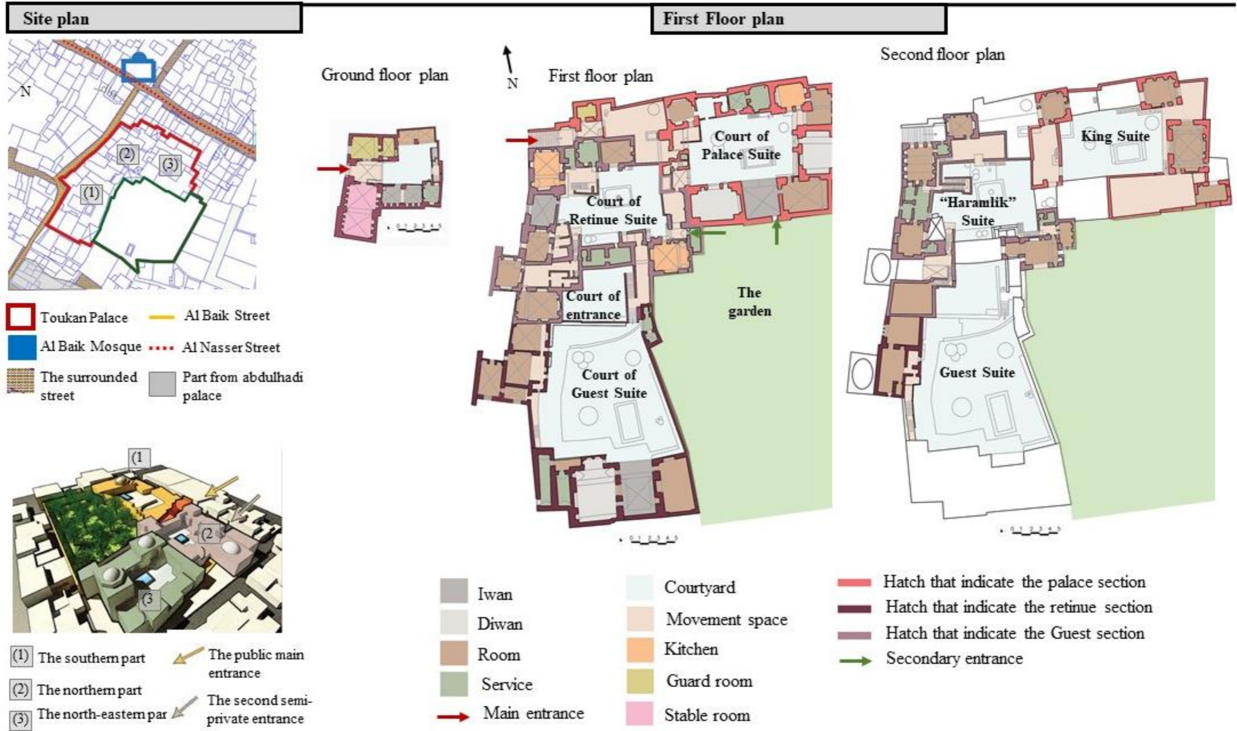
Figure 68: The location and maps with zoning for Toukan palace (Maps from Nablus municipality, editing drawing by author)
