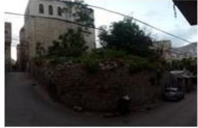
P(12): Blanked elevation with very high opening when the road width and mansion location allow line of sight to reach inner environment
