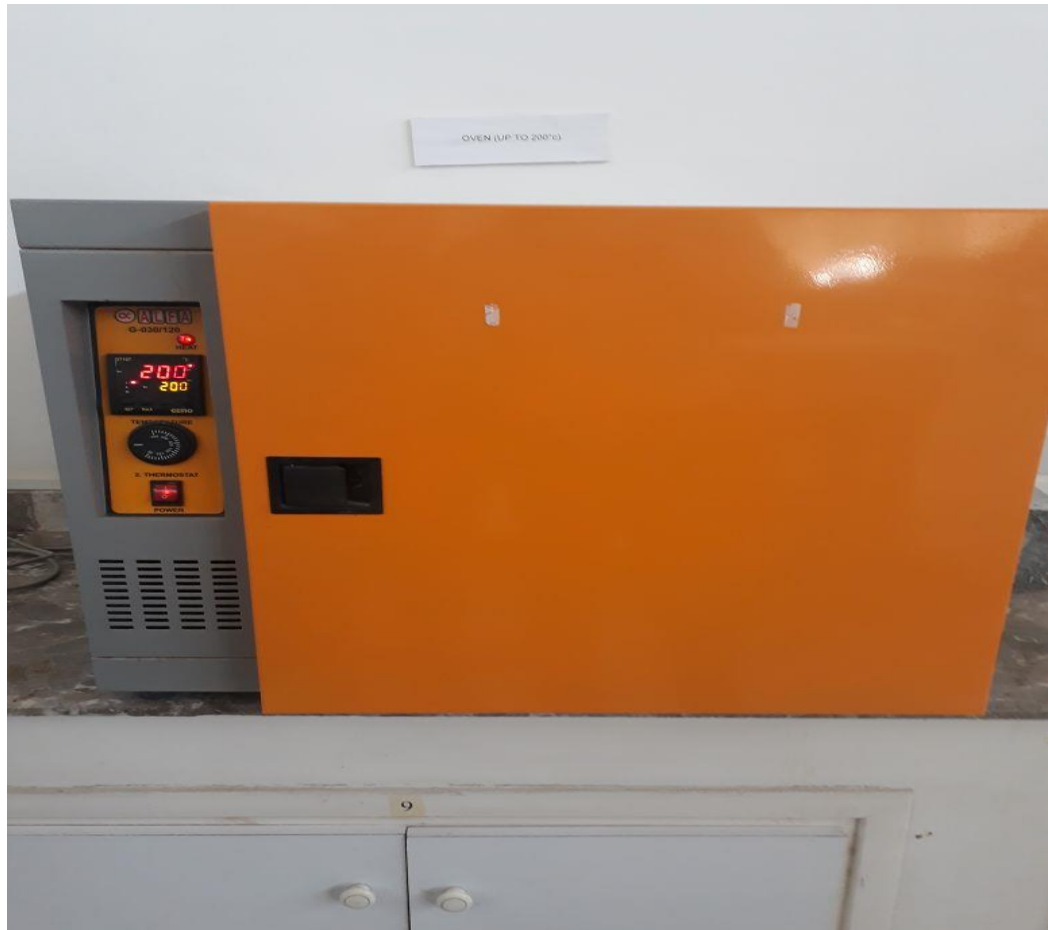
Figure 3.9: Oven Used for Heat Treatment with 200°C Capacity
