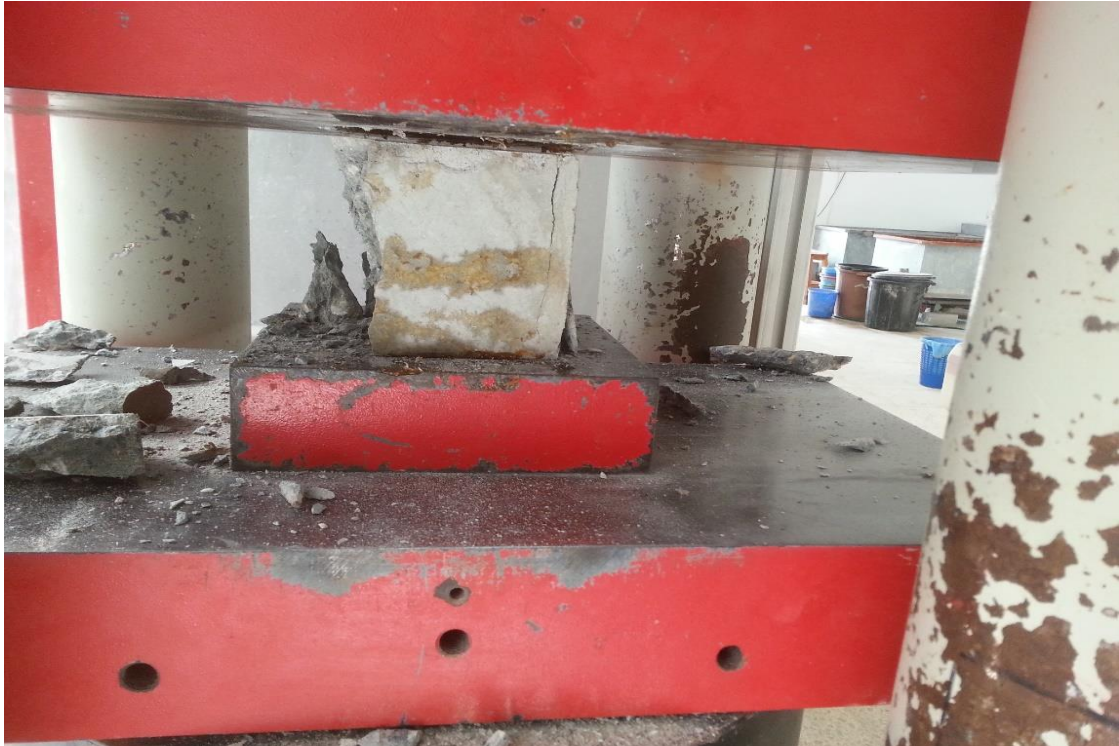
Figure 3.11: Crushed Sample Contained 25% of PP Under Compression Load.
