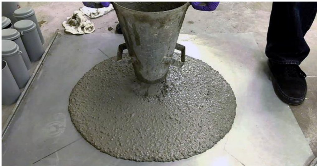
Figure 3.4: slump flow test
