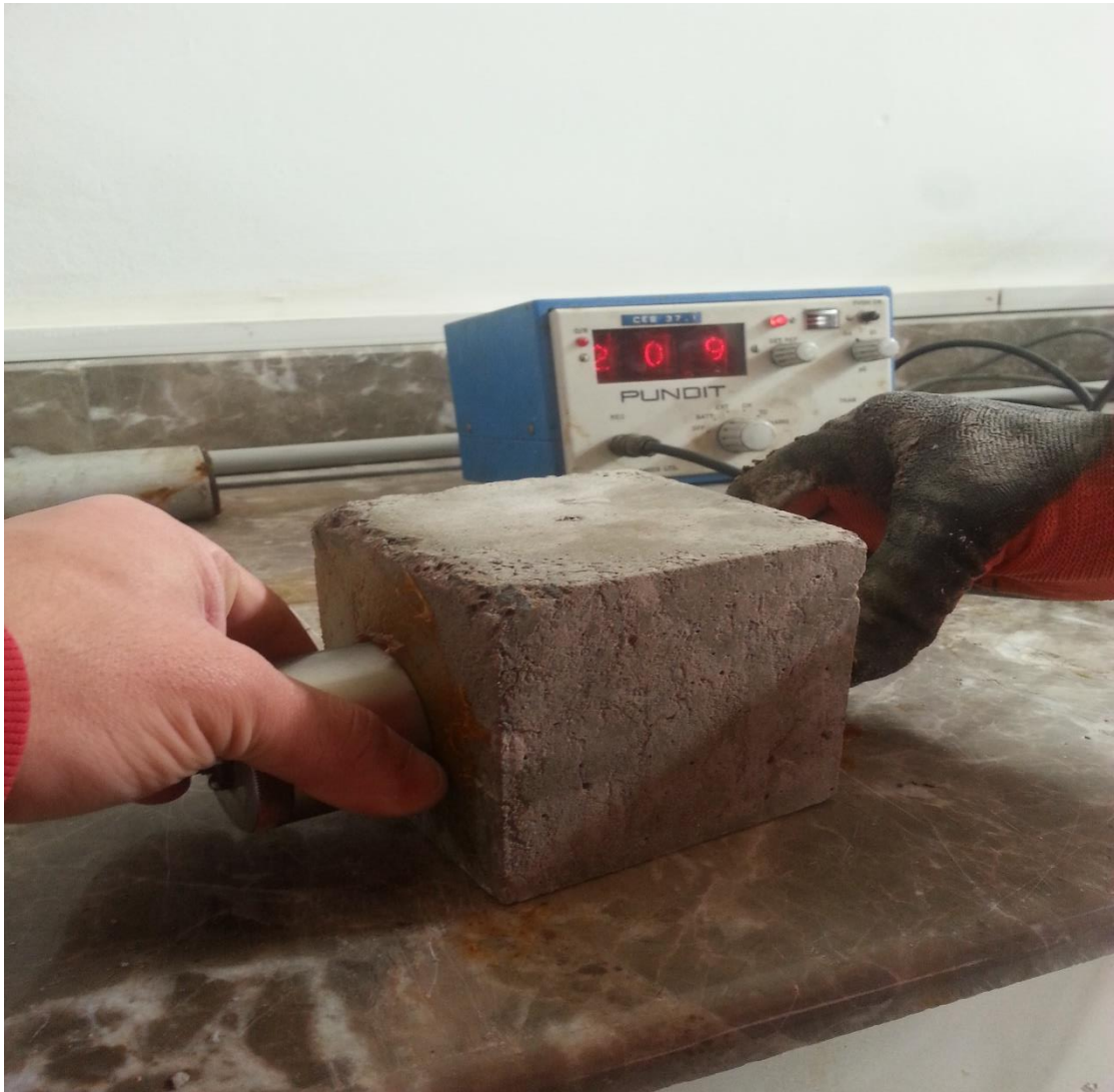
Figure 3.14: Ultrasound Pulse Velocity Measurement
