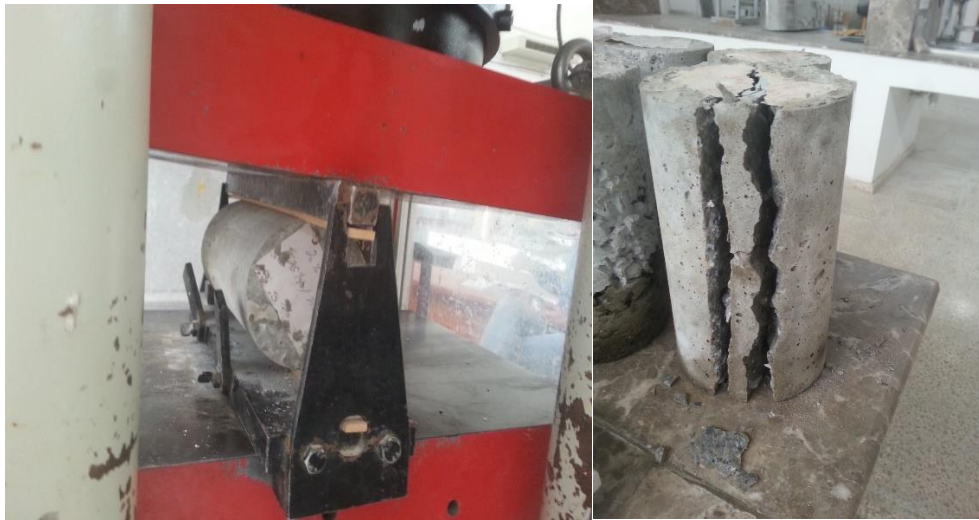
Figure 3.12: Splitting Tensile Test Arrangement and Crushed Specimen.
