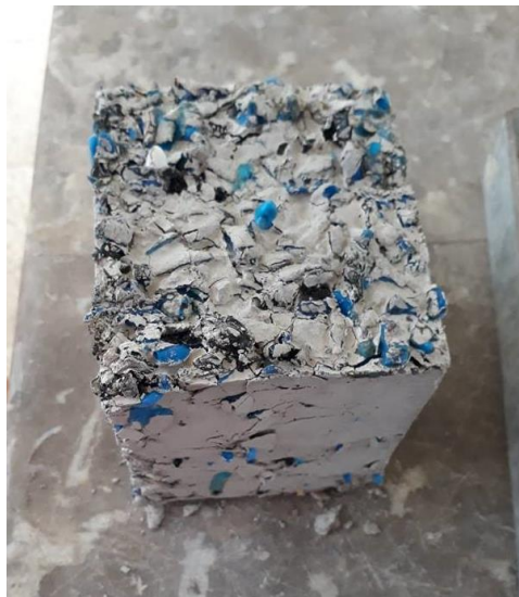
Figure 4.13: SCC30HDPE after Heat Exposure at 200 °C
