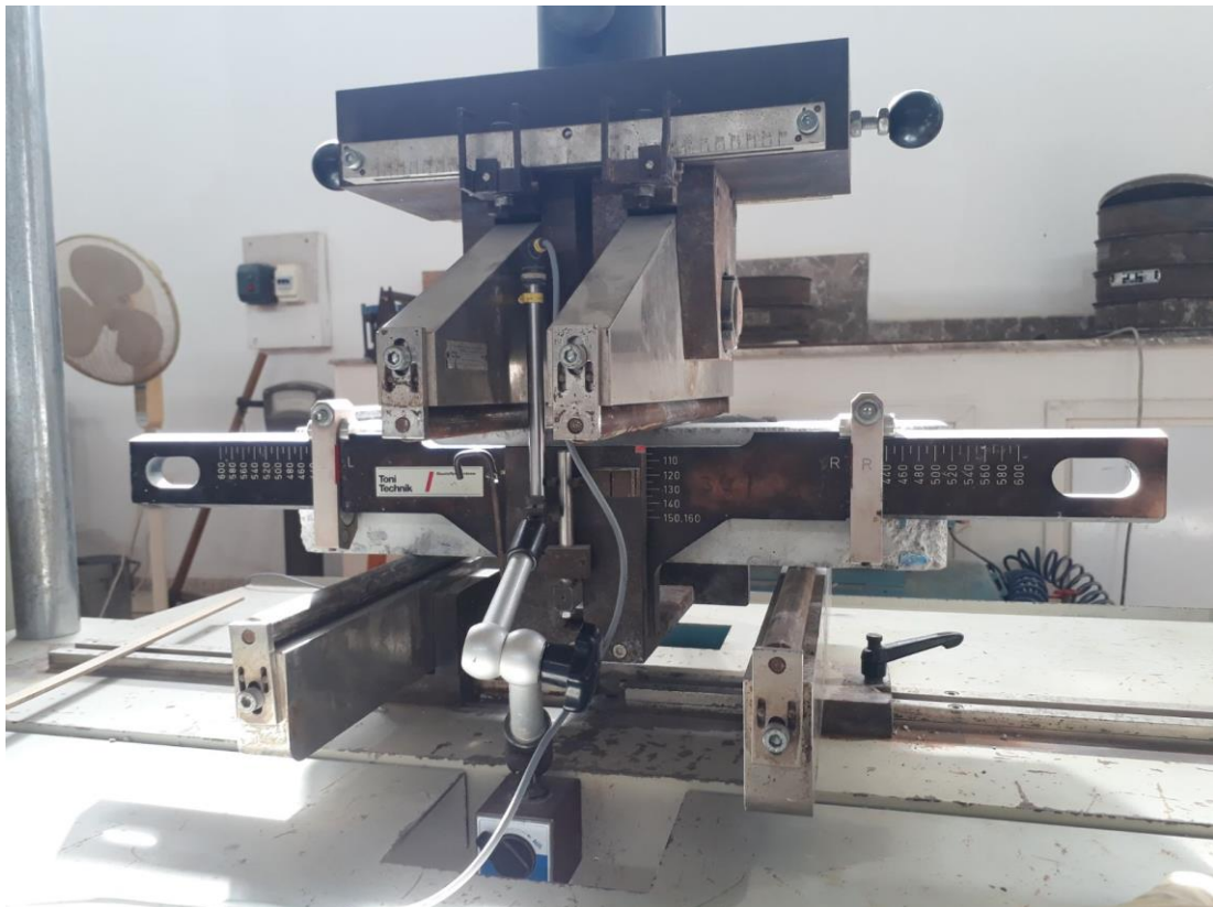
Figure 3.7: Flexural Strength and Toughness Test Arrangement with Yoke
