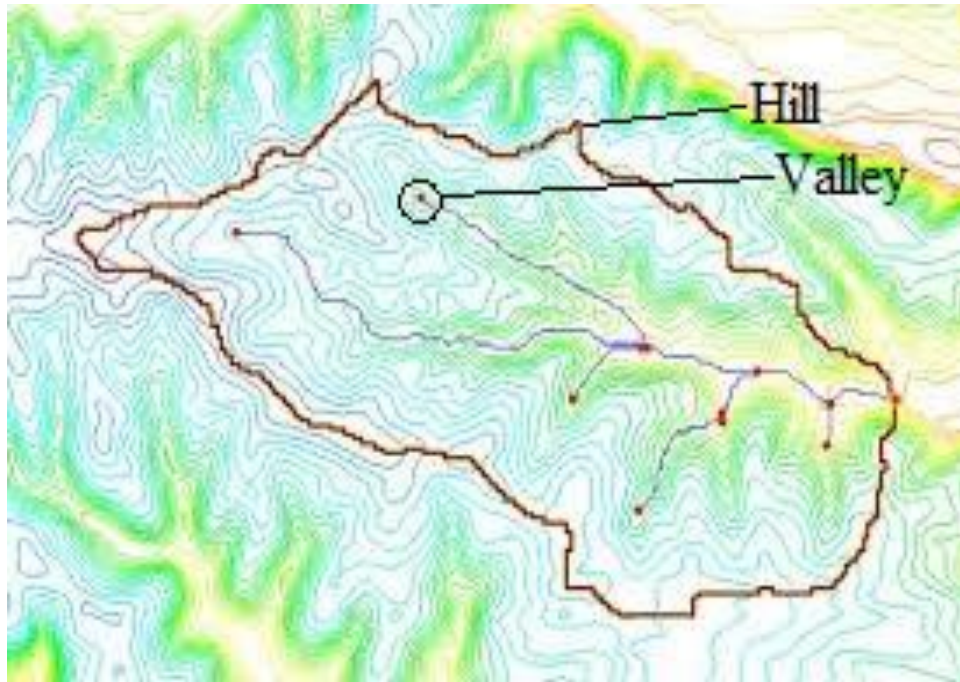
Figure 2.2: Delineating a Watershed Boundary.
