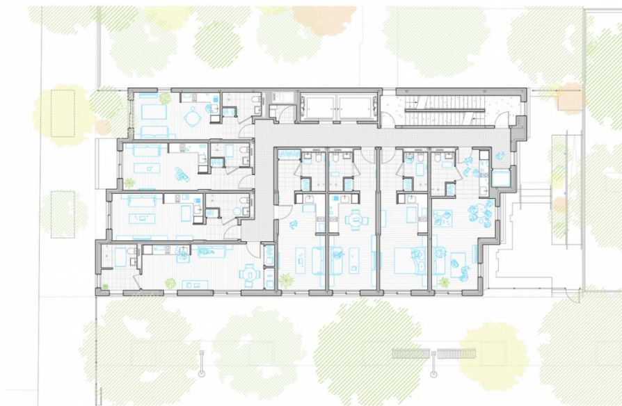
Figure 56: Typical floor plan of Carmel Place shows the 5 different size and orientation in the units per floor. (URL53)
