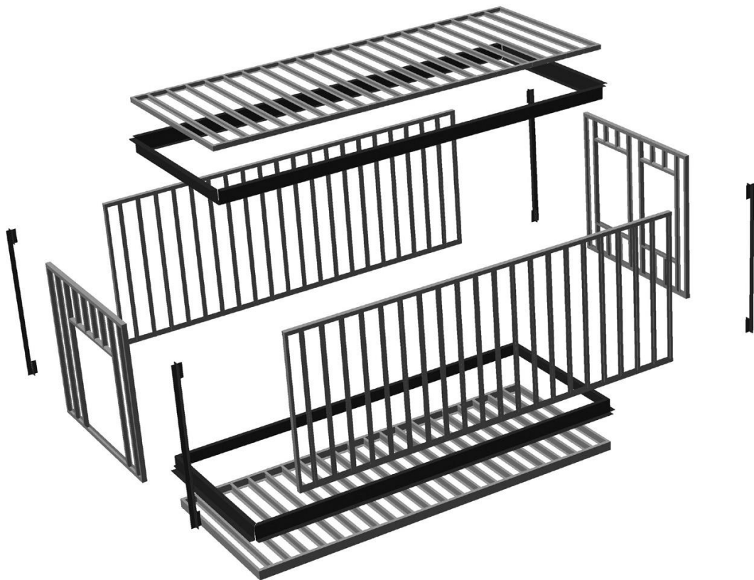
Figure36: Illustration of a four sided module being installed and assembled. (URL40)
