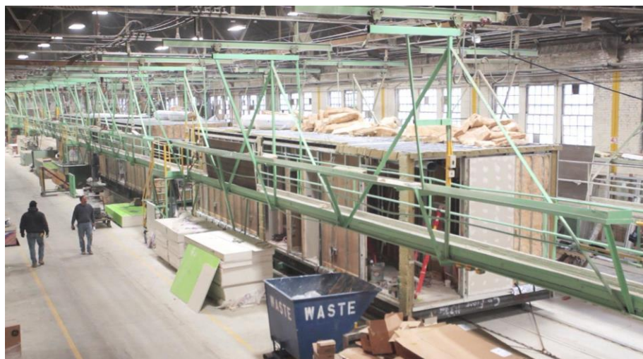
Figure 62: Modules during manufacturing process in the factory (URL56)
