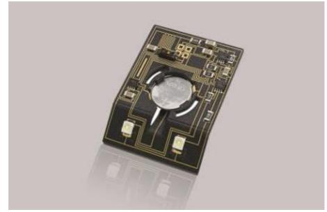
Figure 14: 3D Printed Circuit Board (URL 8)
