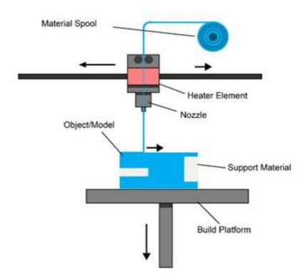
Figure 4: Material Extrusion (URL 2)
