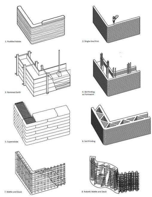
Figure 26: Diagram Comparing Common Building Techniques with Current 3D Printing Processes (URL 21)
